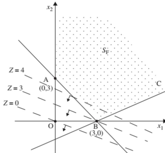
Fig. 2.3 Bounded solutions with unbounded solution space
