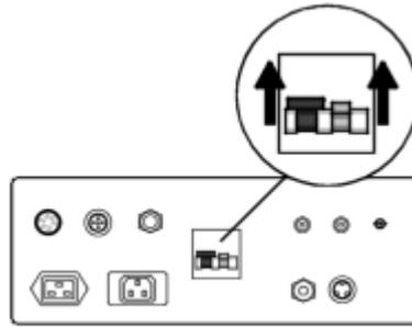
The on/off switch for the apparatus is located on the orange panel on the front of the plinth.
