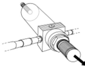
To increase flow through the pressure regulator, turn the knob slowly in a clockwise direction (looking at end of knob). The flow rate is measured by a flow meter downstream of the pressure regulator, and is indicated in L/min on the PCT40 software screen. Flow through the pressure regulator should not be taken above 1.5 L/min as this is the measurement limit of the flow meter. A maximum of 1.4 L/min is recommended.
