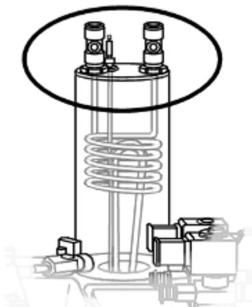
A stainless steel thermometer pocket is located in the lid of the small process vessel. This slows the response of thermocouple T1 when it is inserted into the pocket.
