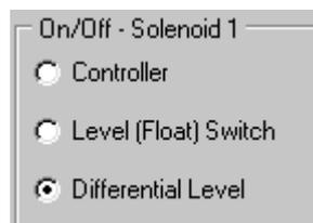
The level in the tank should now be controlled by the differential level switch. SOL 1 should remain open until the water level in the tank reaches the higher of the two electrodes, then close until the water level reaches the lower of the two electrodes.
