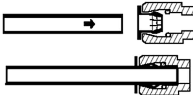
To remove the tube, push the loose circular collet against the body of the Guest push fitting while pulling the tube firmly. The tube will slide out from the fitting. The tube/fitting can be assembled and disassembled repeatedly without damage.
