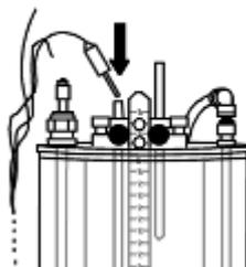
The green plug (green and yellow wire) to the socket on the back of the differential level switch (the connection behind the metal ruler).
