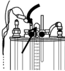
The red plug (brown wire) to the top of the right-hand rod on the differential level switch, which should be positioned to give the high level setpoint.
