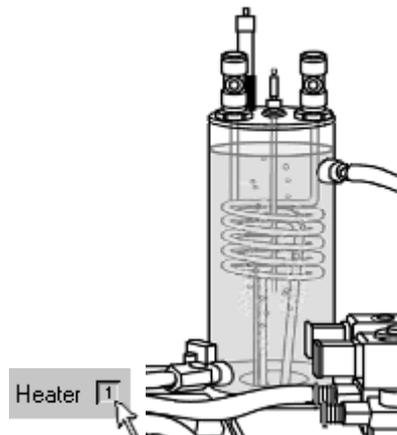
21. Check the temperature sensor readings on the software screen. T1 should increase as the temperature within the vessel rises; T2 and T3 should increase slightly as heat is conducted through the coil.
