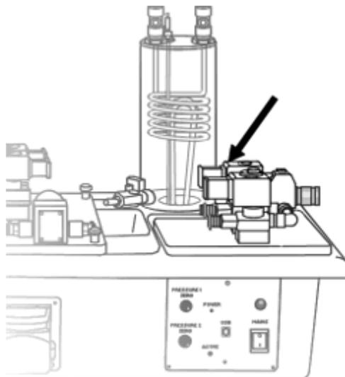
A proportioning solenoid valve is located near the mains water inlet. This is used in some process control exercises to demonstrate proportional control. At other times it may be used to regulate the inlet flow rate.
