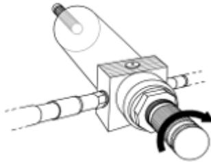
To reduce the flow rate through the pressure regulator, turn the knob slowly in an anticlockwise direction (looking at end of knob):
