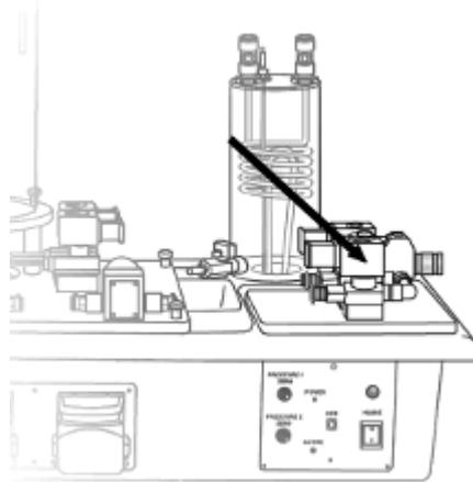
A Normally Closed solenoid valve, SOL 1, is located in front of the Proportioning Solenoid Valve for use in on/off control exercises.
