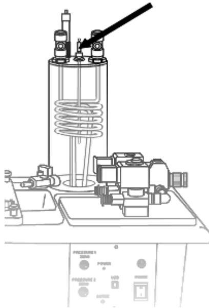
A type k thermocouple temperature probe mounted with the heating/cooling coil in the small process vessel. This probe is used to measure the fluid temperature inside the small process vessel.
