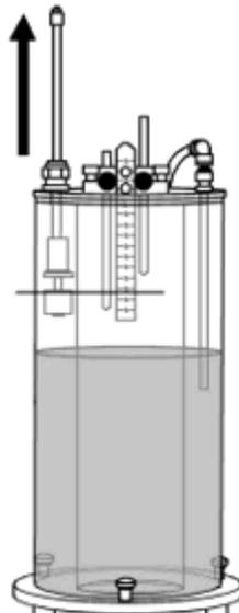
42. Allow the water level to reach the lower electrode on the differential level switch.
