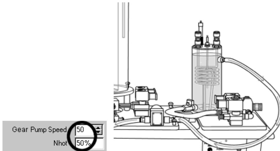
24. When the water level in the small process vessel drops below the tip of the level sensor, the gear pump and the heater should both stop working and the Level Low warning light should turn red. This shows that the safety cut-outs are working.
