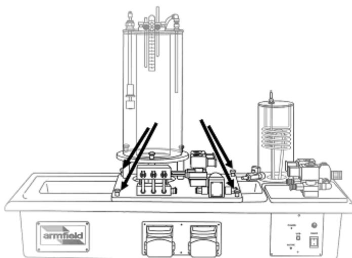
The plinth includes a drainage channel with a drain valve located at the end of the channel. The valve can be connected to a suitable drain using the flexible tubing supplied. The valve should be left open when connected to a drain
