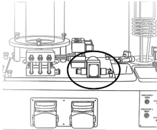
A DC motor-driven pump is located at the front of the plinth. This pump is used to pump hot water during heating and temperature control experiments.
