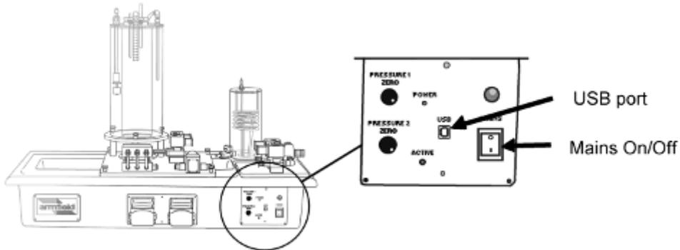
**NOTE:** The red and green LCD indicators on the front of the plinth are associated with the USB connection to the PC. These may be lit even if the PCT40 unit itself is switched off.
