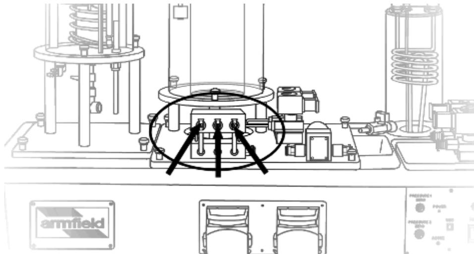
Three piezoelectric differential pressure sensors are located within the bottom section of the manifold block. Each is connected to read the differential pressure across an orifice in the top section of the block. P1 and P2 are small orifices used to measure the small flowrates associated with the optional PCT41. P3 is a large orifice for use with PCT40.
