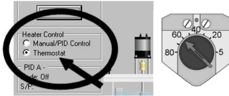
Set the Heater Control back to 'Manual/PID Control'.
