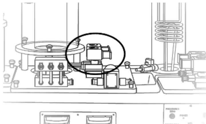
Two Normally Closed solenoid valves, SOL 2 and SOL3, are fitted beneath the large process vessel. The outlet of both valves can be connected to a suitable drain using the flexible tubing supplied.
