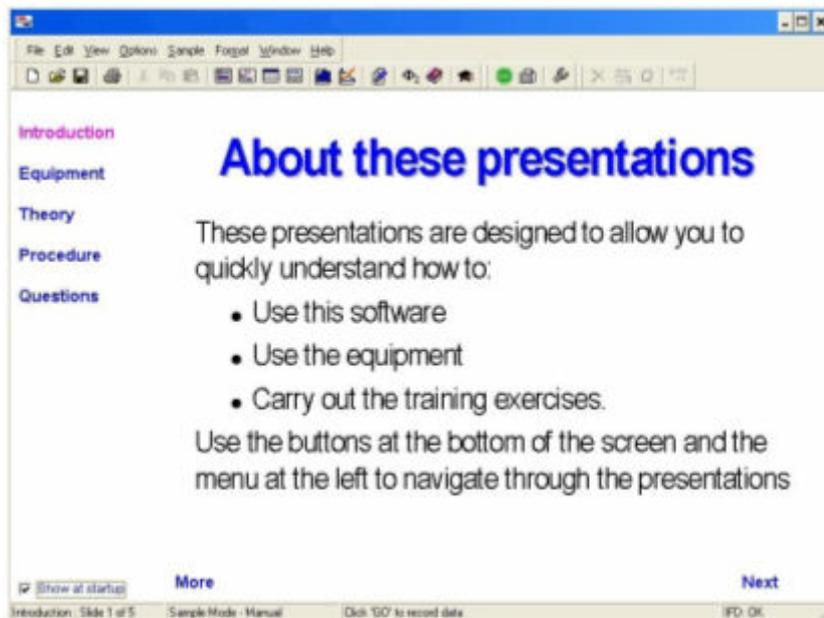
Before proceeding to operate the software ensure that **IFD: OK** is displayed at the bottom of the screen. If IFD:ERROR is displayed check the USB connection between the IFD5 and the PC and confirm that the red and green LED's are both illuminated. If the problem persists then check that the driver is installed correctly (refer to the Operation manual).
