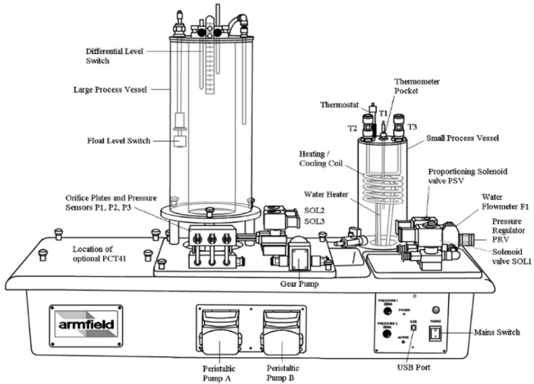
Figure 1 Front View of PCT40
