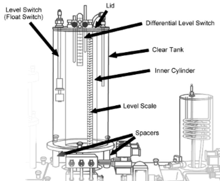
The large acrylic vessel has a removable tube inside to vary the volume of the vessel. When installed on the 'O' rings at the base, the tube creates an annular vessel of reduced volume. The vessel is mounted on spacers to allow access to the connections on the underside. The vessel includes a level scale. Tappings in the base of the vessel allow connections to pressure sensors, solenoid valves and pumps. A vertical overflow tube is included as a safety feature.
