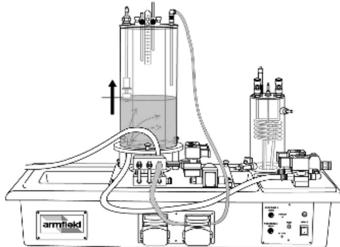
29. Observe that the level sensor reading on the software screen increases as the water level rises. The sensor output should approximately match the level reading from the gauge on the vessel side (the calibration procedure for the sensor is described in the PCT40 software Help Text).
