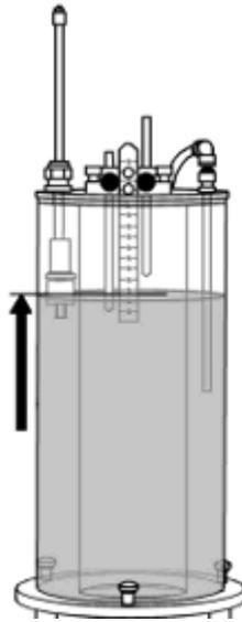
43. Lower the level switch and allow the water level in the vessel to drop to 50mm below the level of the differential level sensor.
