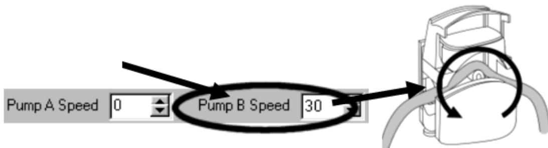
32. With the pump running, close the pump lid. Water should now be drawn along the tube from the large process vessel, through the pump and then through the differential pressure sensor set within the manifold block (in front of the large process vessel).
