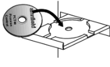
Insert the PCT40 software CD-ROM into the CD-R drive of a suitable PC. The installation program should autorun. If it does not, select 'Run...' from your Start menu, type run d:\setup where d is the letter of your CD-ROM drive. Follow the instructions on screen.
