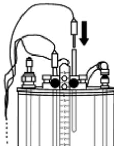
41. Adjust the level switch (float switch) until the float is higher than the lower of the two electrodes on the differential level switch.
