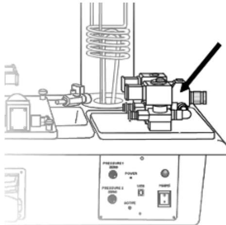
The mains water inlet is connected to a pressure regulating valve with integral filter. The flow of water through the equipment can be varied by adjusting the setting of the regulator.
