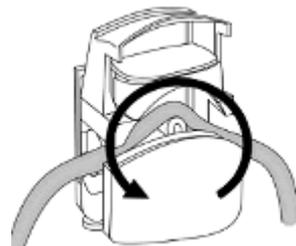
36. Close the pump lid. Water should now be drawn along the flexible tubing from the large process vessel, through Pump A and the differential pressure sensor then out to drain.
