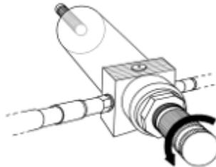
Once the appropriate flow rate is achieved, lock the regulator setting by pushing the grey knob back towards the body of the regulator:
