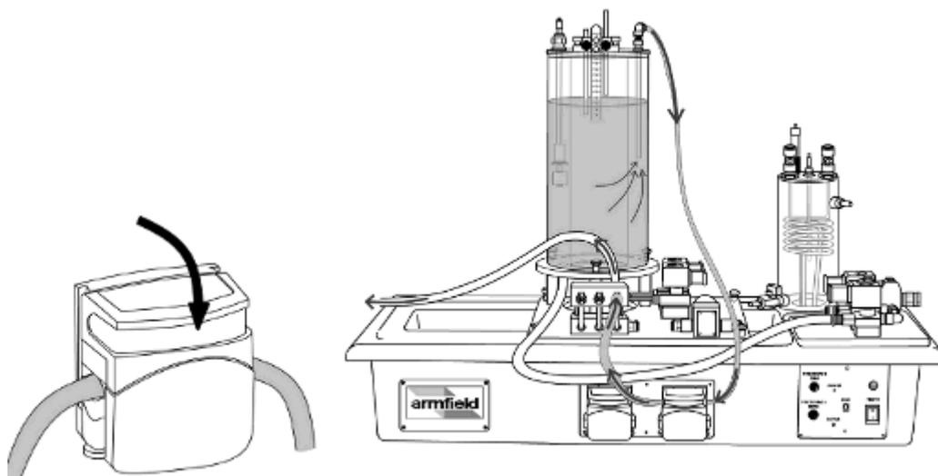
33. Check that there is a positive reading from the differential pressure sensor P3. Increase the speed of Pump B, and check that the differential pressure reading also increases. Reduce the speed of Pump A to 0.
