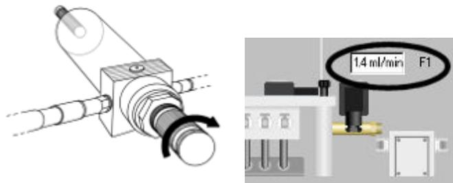
17. Lock the regulator setting by pushing the grey knob back towards the body of the regulator:
