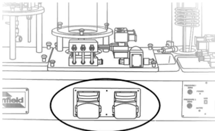
Two identical peristaltic pumps are located on the front of the plinth. These can take a wide range of silicone tubing, examples of which are included with the apparatus. The pumps may be operated individually or in parallel according to the control exercise. Pump A is located on the left-hand side, Pump B is located on the right-hand side.
