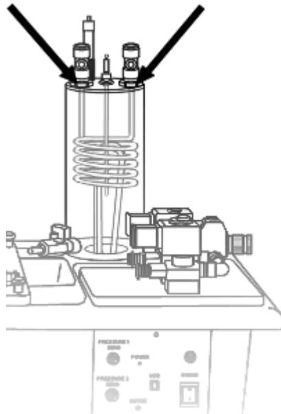
Two type K thermocouples located at the inlet and the outlet of the heating/cooling coil. These are used to measure the temperature of the fluid as it enters and leaves the coil.
