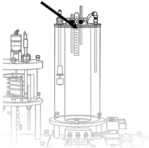
A variable dead-band conductive level switch consisting of fixed earth rod and adjustable high / low level electrodes on a support.
