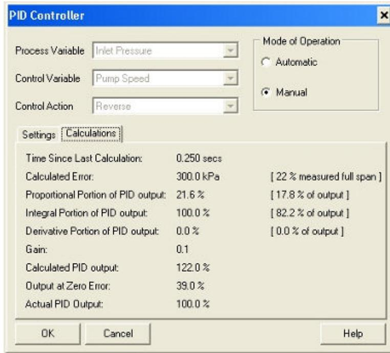
The Mode of operation always defaults to **Manual** control and 0% output when the software is loaded to ensure safe operation of the equipment. If appropriate, the operator can retain manual operation and simply vary the value from 0 to 100% in the **Manual Output** box, then clicking **Apply**.
