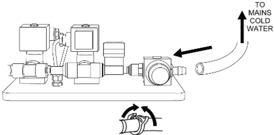
4. Connect the tubing supplied with right-angle (90°) Guest push fittings to the valves SOL2 and SOL3 beside the large process vessel.
