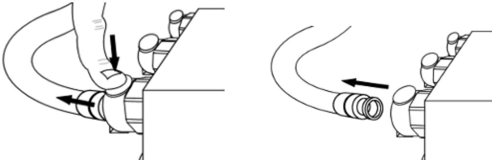
Where appropriate, some quick release fittings incorporate a self-sealing valve to prevent loss of fluid when the fitting is disconnected.
