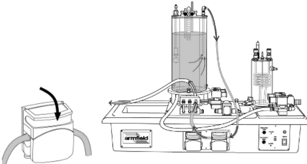
37. Vary the pump speed using the arrow keys to check that the pump is controlling correctly, then set the pump speed back to 0%.
