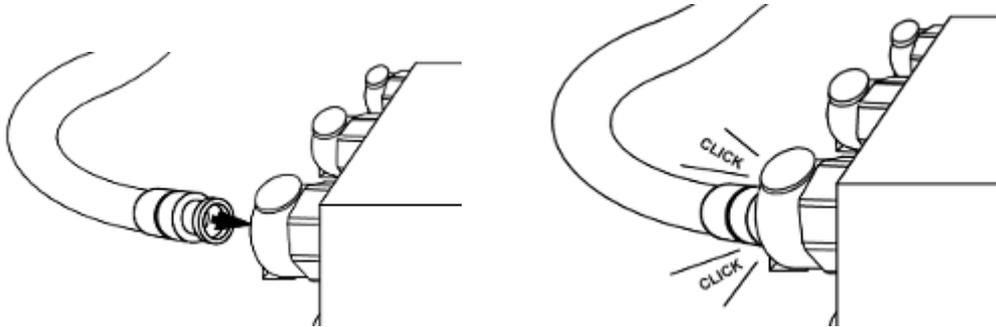
To remove a tube, press the metal catch against the socket and pull the tube free.
