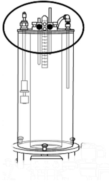
The lid of the vessel supports an adjustable height level switch, a differential level switch and a dip tube for filling or draining the vessel from the top using one of the pumps or control valves.
