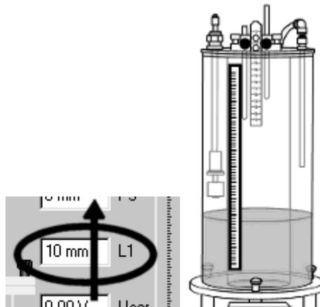
30. Allow the water in the large process vessel to reach a level of 250mm, then close the valve SOL1 by setting it back to 0%.
