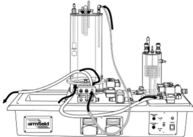
26. Insert the soft silicone tubing into the peristaltic pump as shown.
