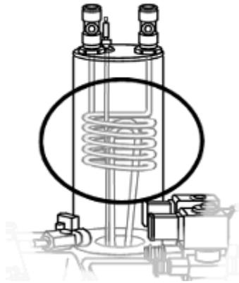
This is a stainless steel coil mounted on a lid that is designed to fit inside the small process vessel around heating element. Fittings at the inlet and outlet of the coil accommodate thermocouple-type temperature sensors and allow connection to the water supply.
