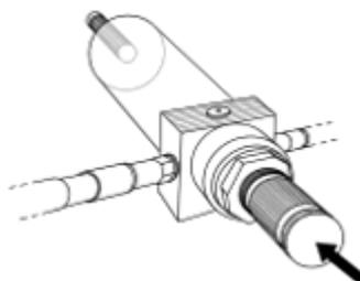
18. Alter the setting of the PSV using the arrow keys. Flow into the small process vessel should increase as the valve setting increases, and decrease as the setting decreases. After testing, set the valve to 50% until the small process vessel fills and water covers the tip of the level sensor.
