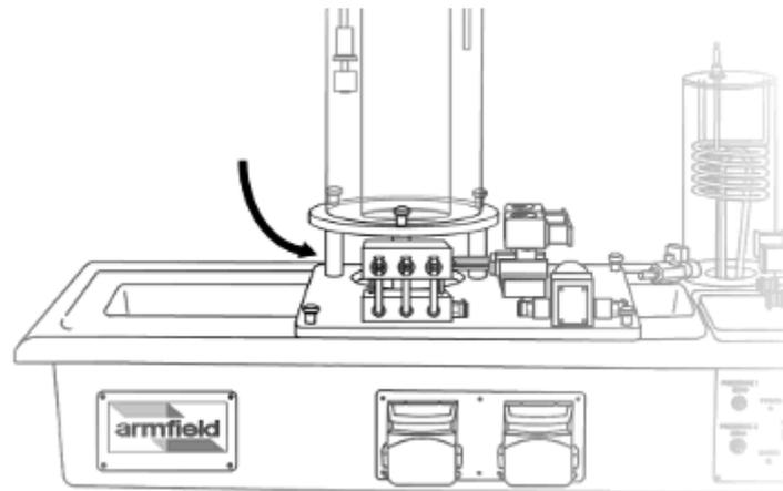
A type K thermocouple is located near the back of the base plate to the left of the large process vessel. This sensor is used during experiments utilising a holding tube, to measure fluid temperature at the outlet of the holding tube. This sensor is also used to measure temperature inside the reactor of the optional PCT41.
