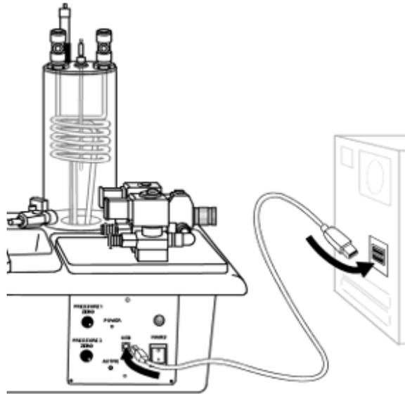
9. The computer should automatically detect the USB interface device. Follow the instructions to install the correct driver:
