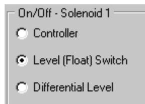
SOL1 should open when the water level in the tank drops so that the float reaches its lowest position...
