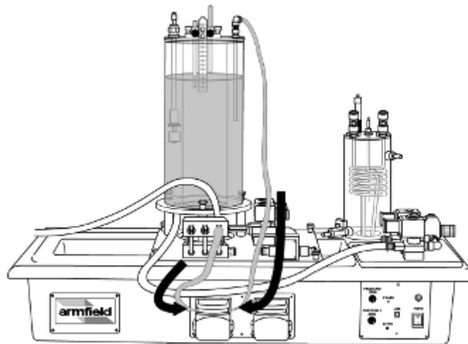
35. With Pump A open, set the speed of the pump to 30%. The pump should begin to operate.
