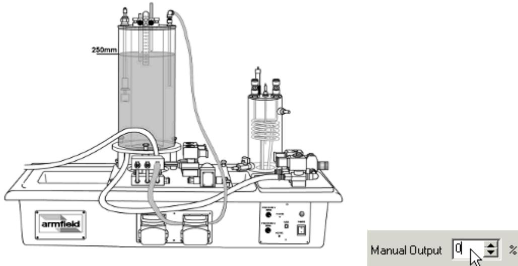
31. With the lid of the pump still open, set the speed of the pump to 30% by typing this value into the display box on the software screen. The pump should begin to operate.
