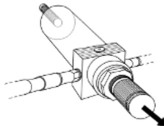
16. Turn the knob slowly in a clockwise direction (looking at end of knob) to set a flow rate of 1.4 L/min.
