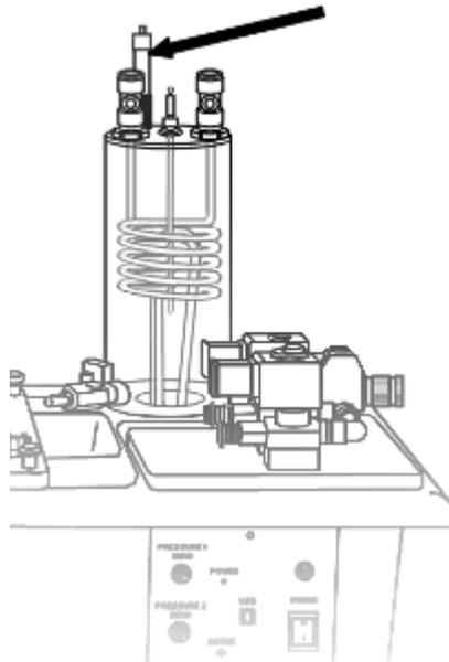
A fixed dead-band temperature switch consisting of a rod thermostat with adjustable set point.
