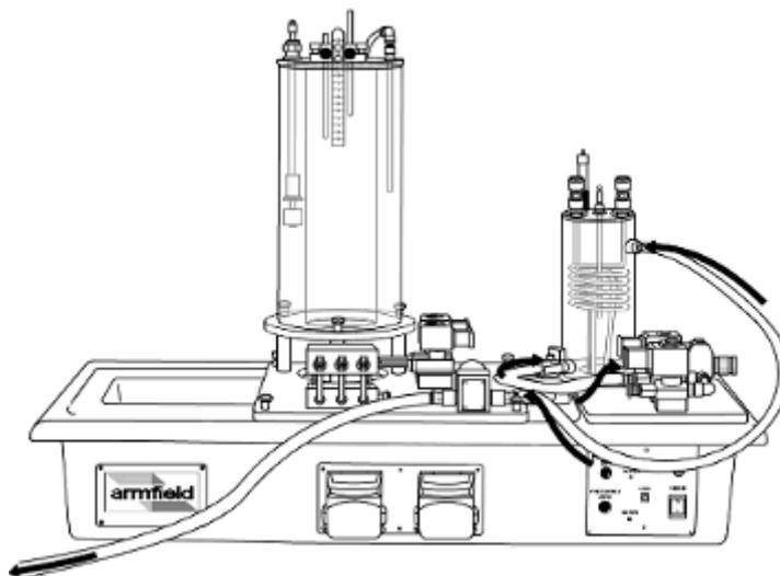
13. Close the pressure regulator: pull the grey knob away from the body of the regulator, turn the knob fully anticlockwise, then push the knob back in.
