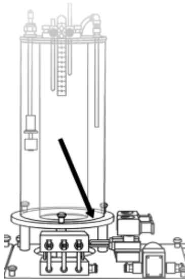
A piezoelectric pressure sensor is mounted in the base of the large process vessel. One side is connected to the inside of the process vessel, and the other is open to atmosphere, allowing the pressure in the process vessel to be measured relative to atmosphere. This sensor therefore measures the level of water in the vessel.
