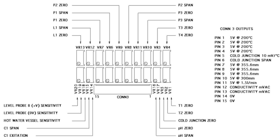
**Note:** The software supplied with the PCT40 includes the ability to recalibrate each of the sensors if necessary. Small changes in calibration should therefore be made using the software. Re-calibration using the potentiometers should not therefore be necessary unless a large change is required such as following the replacement of a sensor etc.
