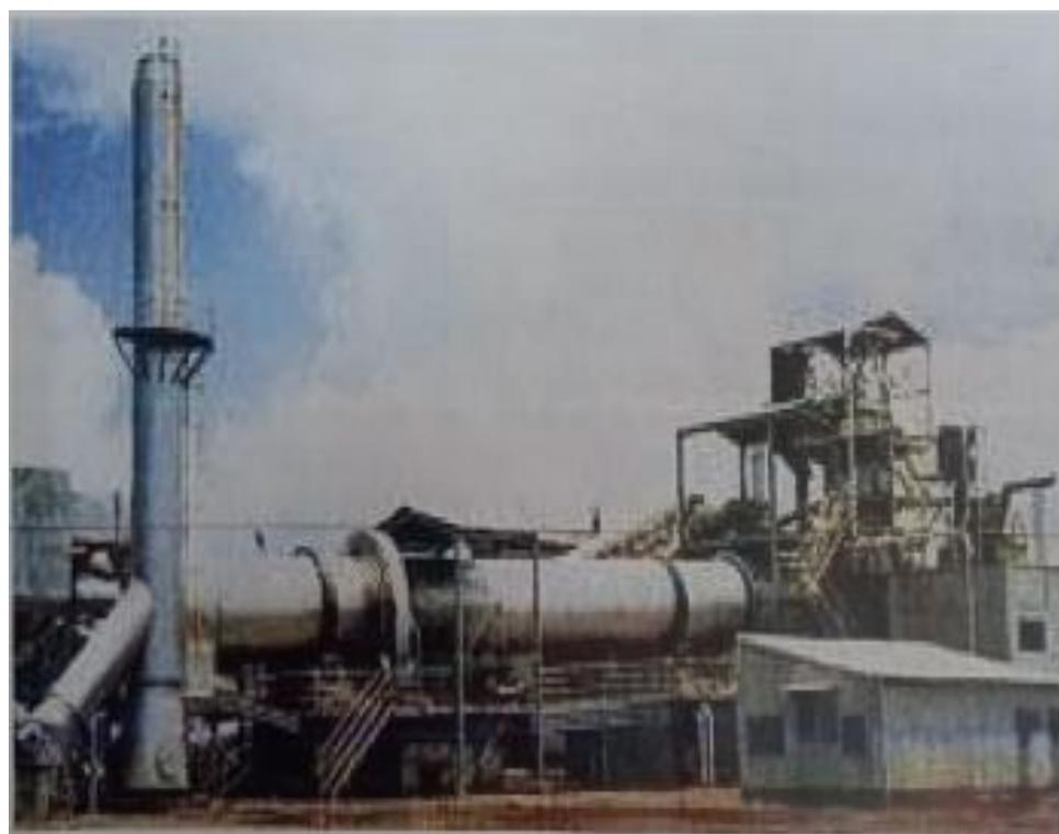
Figure 4. Rotary kiln used in manufacturing of cement
