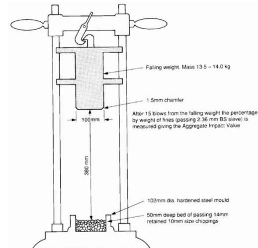
Figure 1. Apparatus for the aggregate impact test (Millard, 1993)
