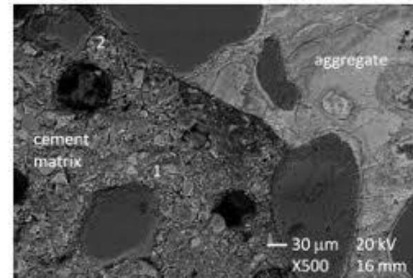
Figure 5. SEM-BSE analyses of concrete 1 (without doping).
