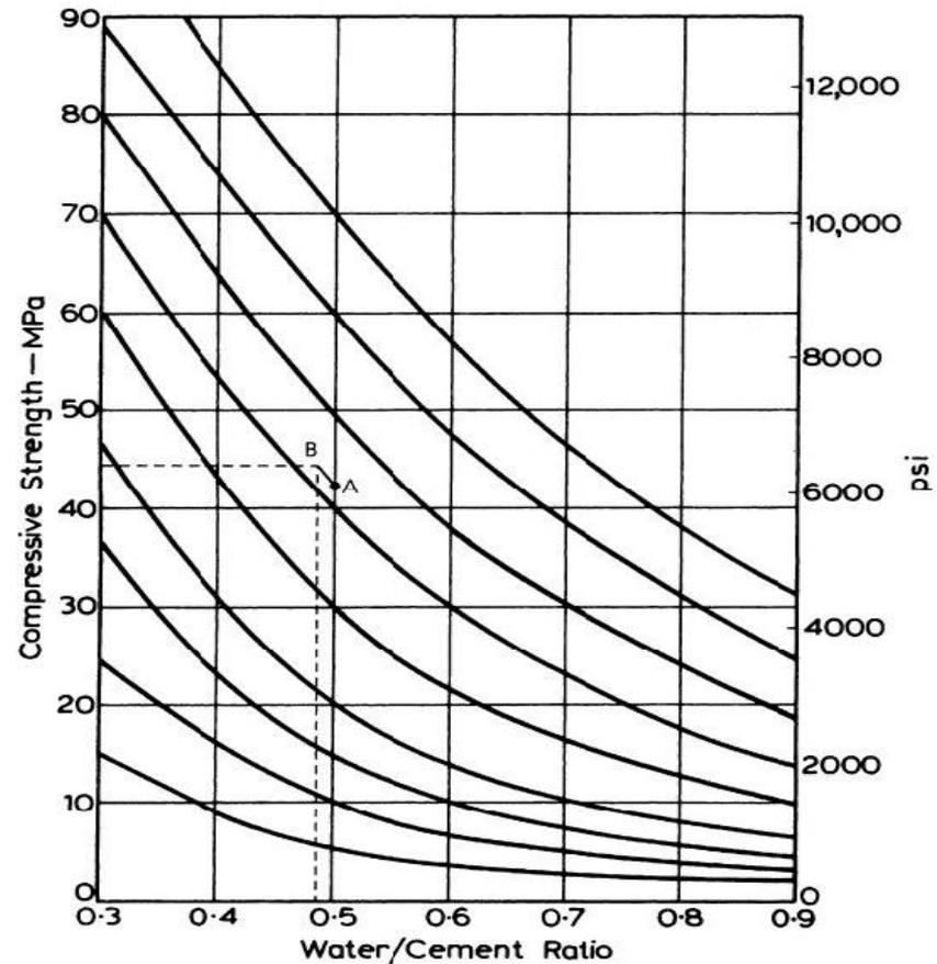
Fig. 1, Relation between compressive strength and free water/cement ratio for use in the British mix selection method.
