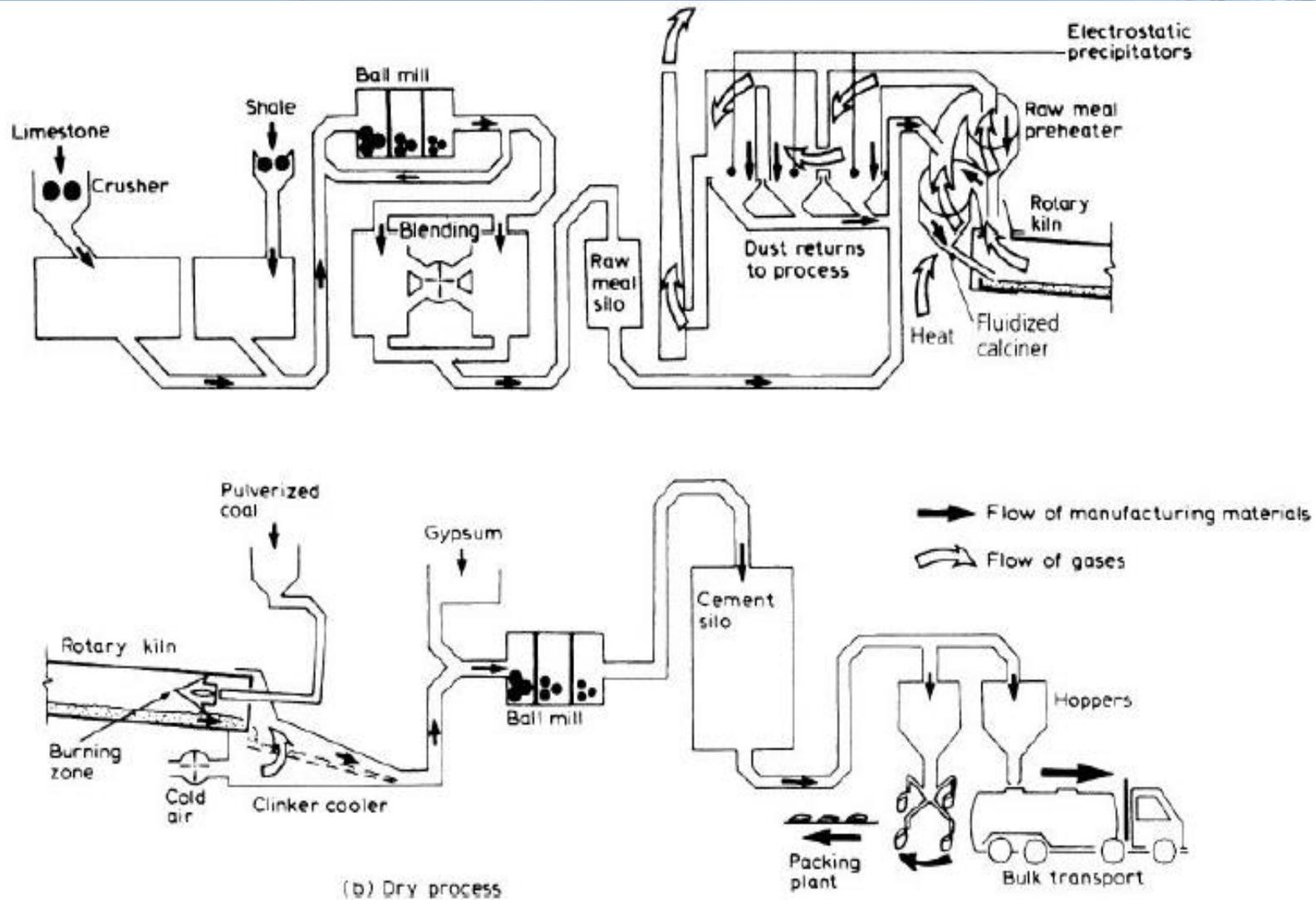
Fig. 1.1. Diagrammatic representation of: (a) the wet process and (b) the dry process of manufacture of cement
