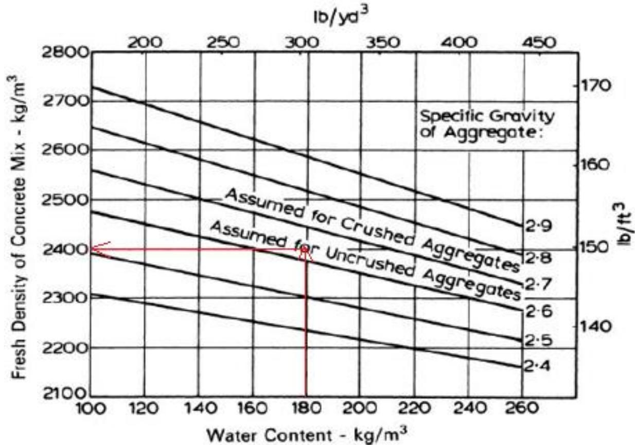
Fig. 2, Estimated wet density for fully compacted concrete (specific gravity is given for saturated and surface-dry aggregate)
