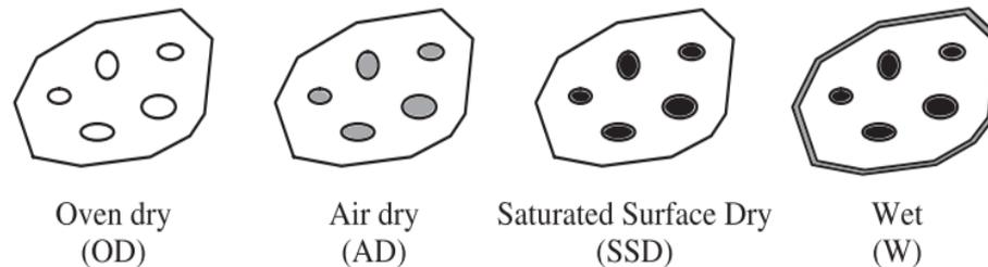
Figure. Aggregate in various moisture states
