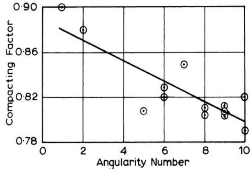
Figure. The relation between the angularity number of aggregate and the compacting factor of concrete
