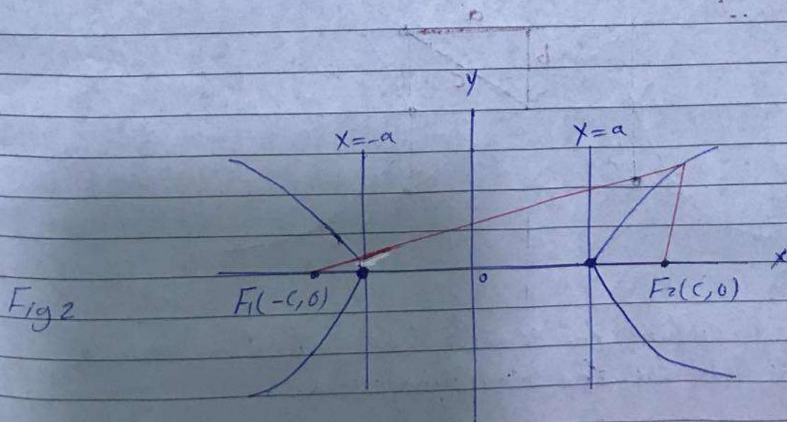
It is traditional in the study of hyperbolas to denote the distance between the vertices by  $2a$ , the distance between the foci by  $2c$ . Figure 3, and to define the quantity  $b$  as  $b = \sqrt{c^2 - a^2}$ . This relationship, which can also be expressed as
