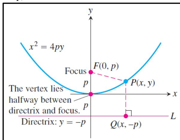
In the notation of the figure, a point  $P(x, y)$  lies on the parabola if and only if  $PF = PQ$ . From the distance formula,
