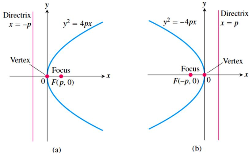
(a) The parabola  $y^2 = 4px$  (b) The parabola  $y^2 = -4px$ .
