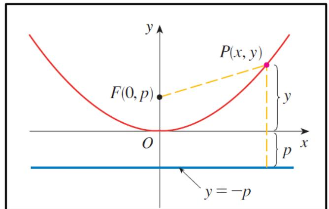
A parabola has its simplest equation when its focus and directrix straddle one of the coordinate axes. For example, suppose that the focus lies at the point  $F(0, p)$  on the positive  $y$ -axis and that the directrix is the line  $(y = -p)$
