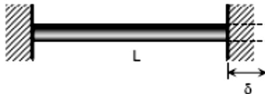
Deformation due to temperature changes;
