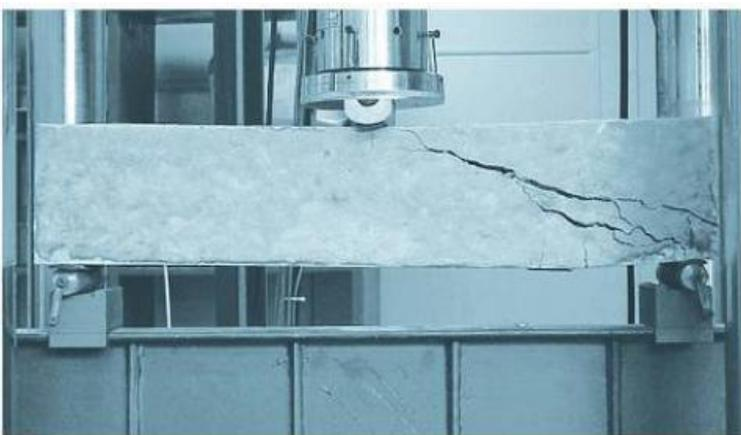
The cracks in this concrete beam were caused by tension stress, even though the beam was subjected to both an internal moment and shear. The stress transformation equations can be used to predict the direction of the cracks, and the principal normal stresses that caused them.
