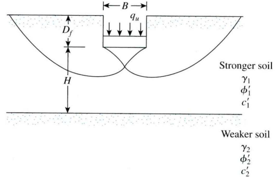
$$q_u = q_b + \frac{2c_a \times H}{B} + \gamma_1 H^2 \left(1 + \frac{2D_f}{H}\right) \times \frac{K_s \tan \phi_1}{B} - \gamma_1 \times H$$
