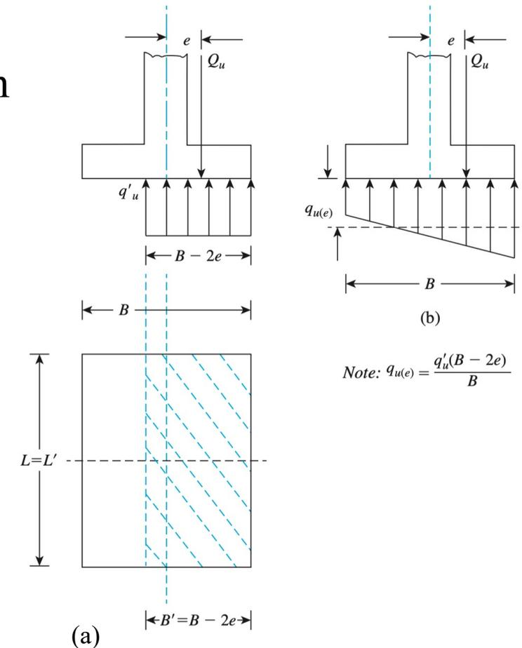
**Example:** A continuous (strip) foundation is shown in the Figure. If the load eccentricity is 0.2 m, determine the ultimate load,  $Q_u$ , per unit length of the foundation. Use Meyerhof's effective area method.
