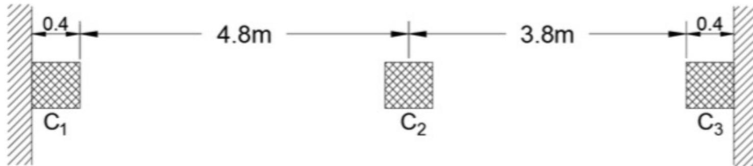
**B.** Design a combined footing for the same figure above if  $C_1$  has a dead load of 90 tons and live load of 54 tons, knowing that the extension is not permitted and the soil reaction is being uniform. ( $q_{all,net} = 20.8 \text{ t/m}^2$ ).
