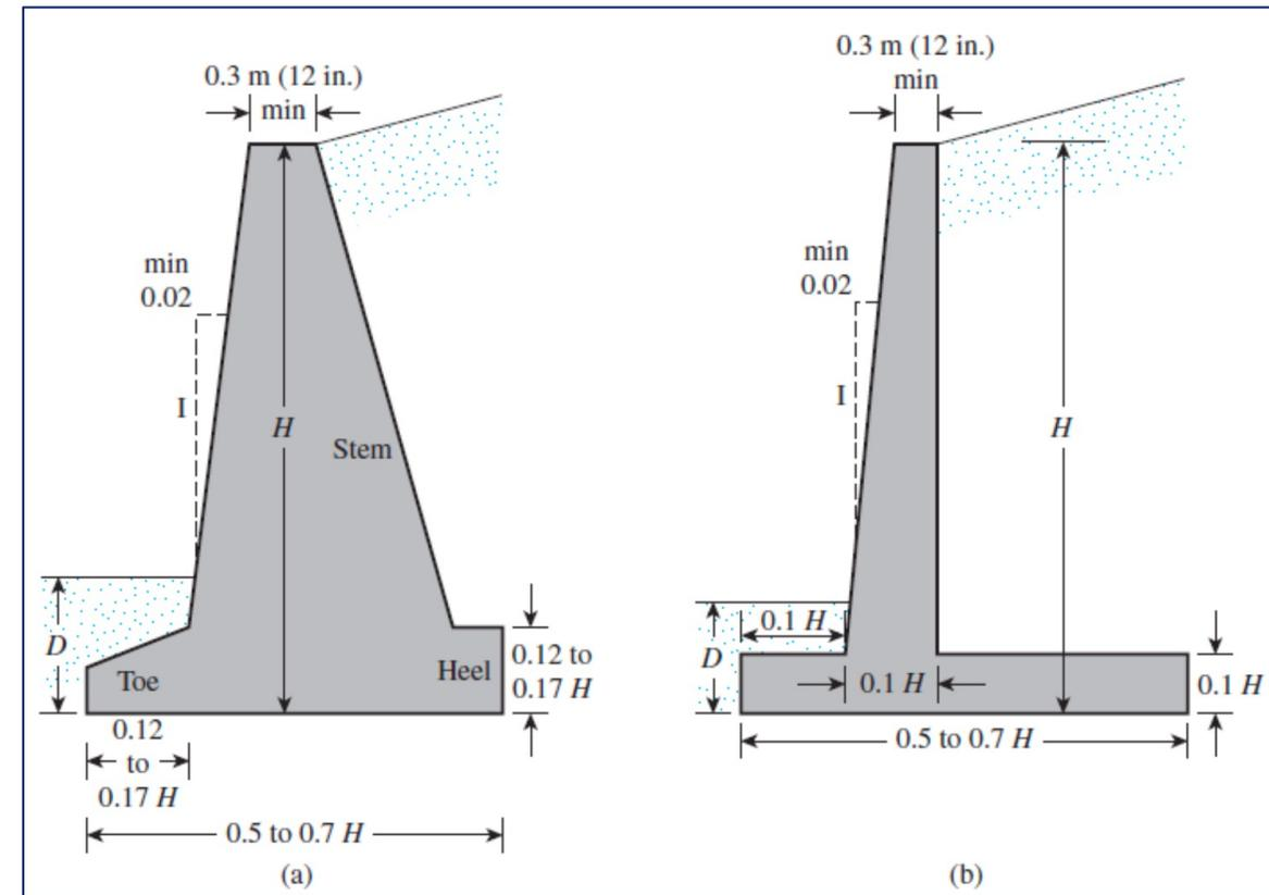
(a): Gravity wall, (b): Cantilever wall
