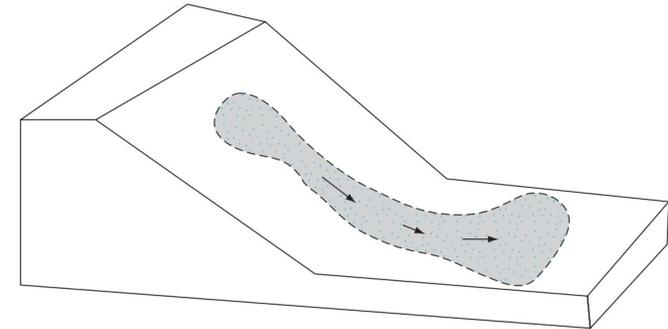
5: Slope failure by "flowing"
