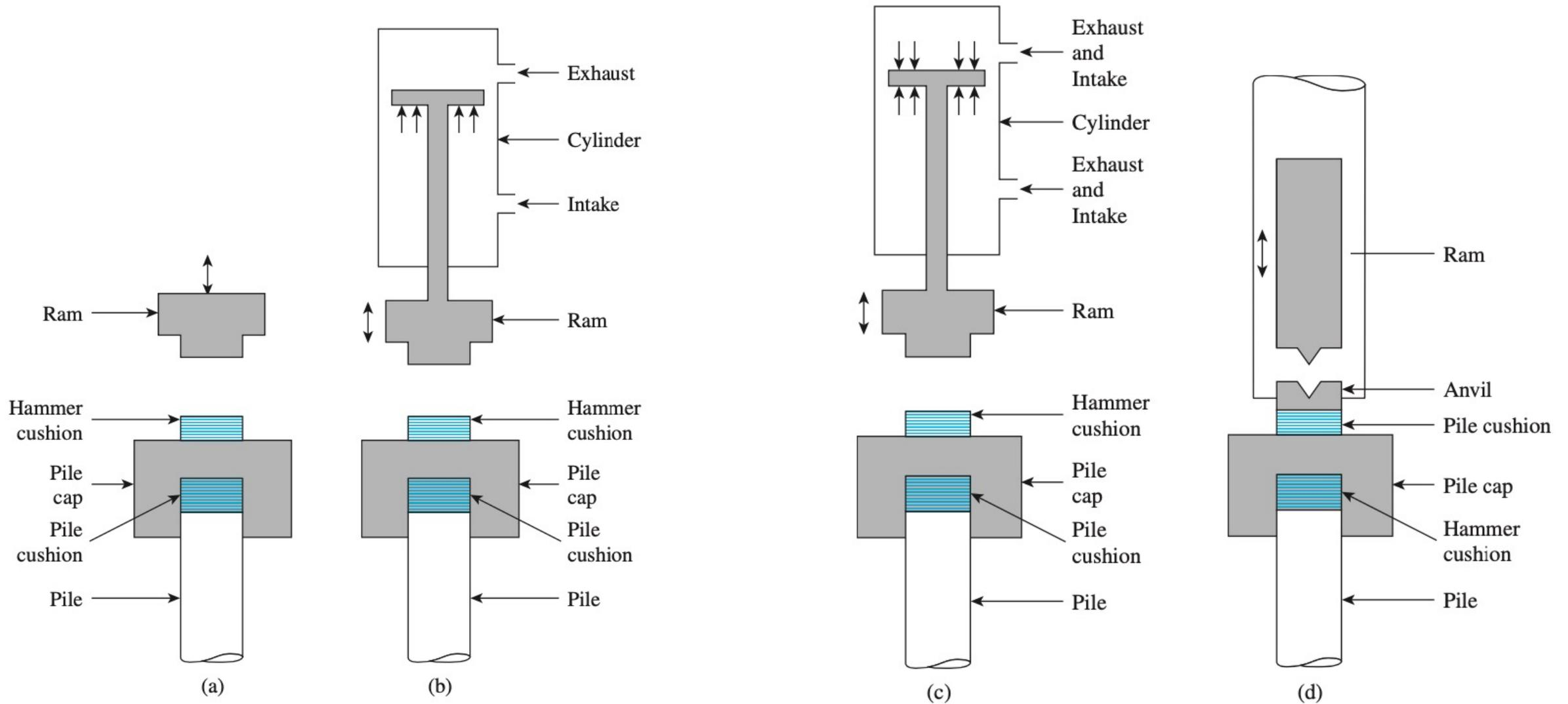
Pile-driving equipment: (a) drop hammer; (b) single-acting air or steam hammer; (c) double-acting and differential air or steam hammer; (d) diesel hammer
