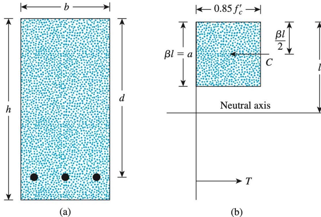
$\beta = 0.85$  for  $f'_c$  of  $28 \text{ MN/m}^2$  ( $4000 \text{ lb/in.}^2$ ) or less and decreases at the rate of 0.05 for every  $7 \text{ MN/m}^2$  ( $1000 \text{ lb/in.}^2$ ) increase of  $f'_c$ . However, it cannot be less than  $0.65$  in any case (ACI Code Section 10.2.7).
