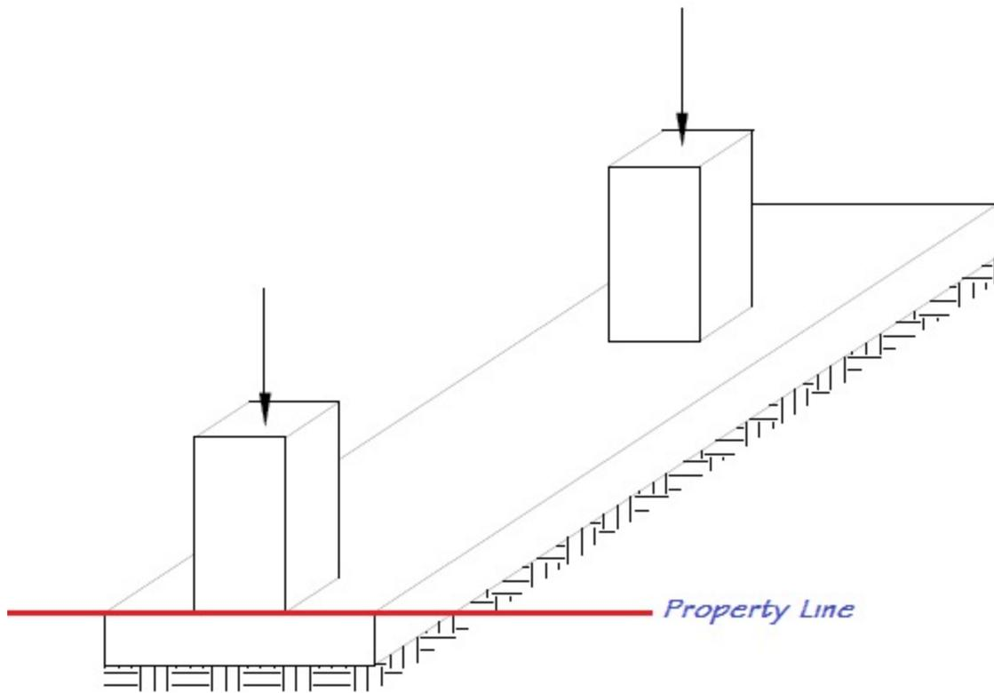
**A third case of a useful application of a combined footing is if one (or several) columns are placed right at the property line. The footings for those columns can not be centered around the columns. The consequent eccentric load would generate a large moment in the footing. By tying the exterior footing to an interior footing through a continuous footing, the moment can be substantially reduced, and a more efficient design is attained.**
