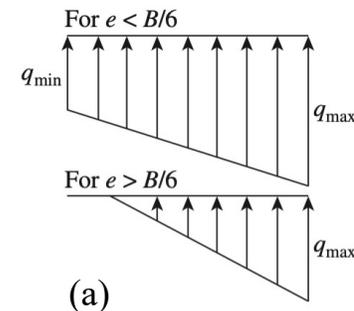
Substituting Equation of (e) into Eqs. of  $q_{\max}$  and  $q_{\min}$  gives
