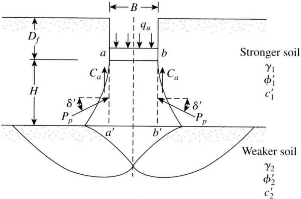
If the depth  $H$  is relatively large (thickness of top layer is large)
