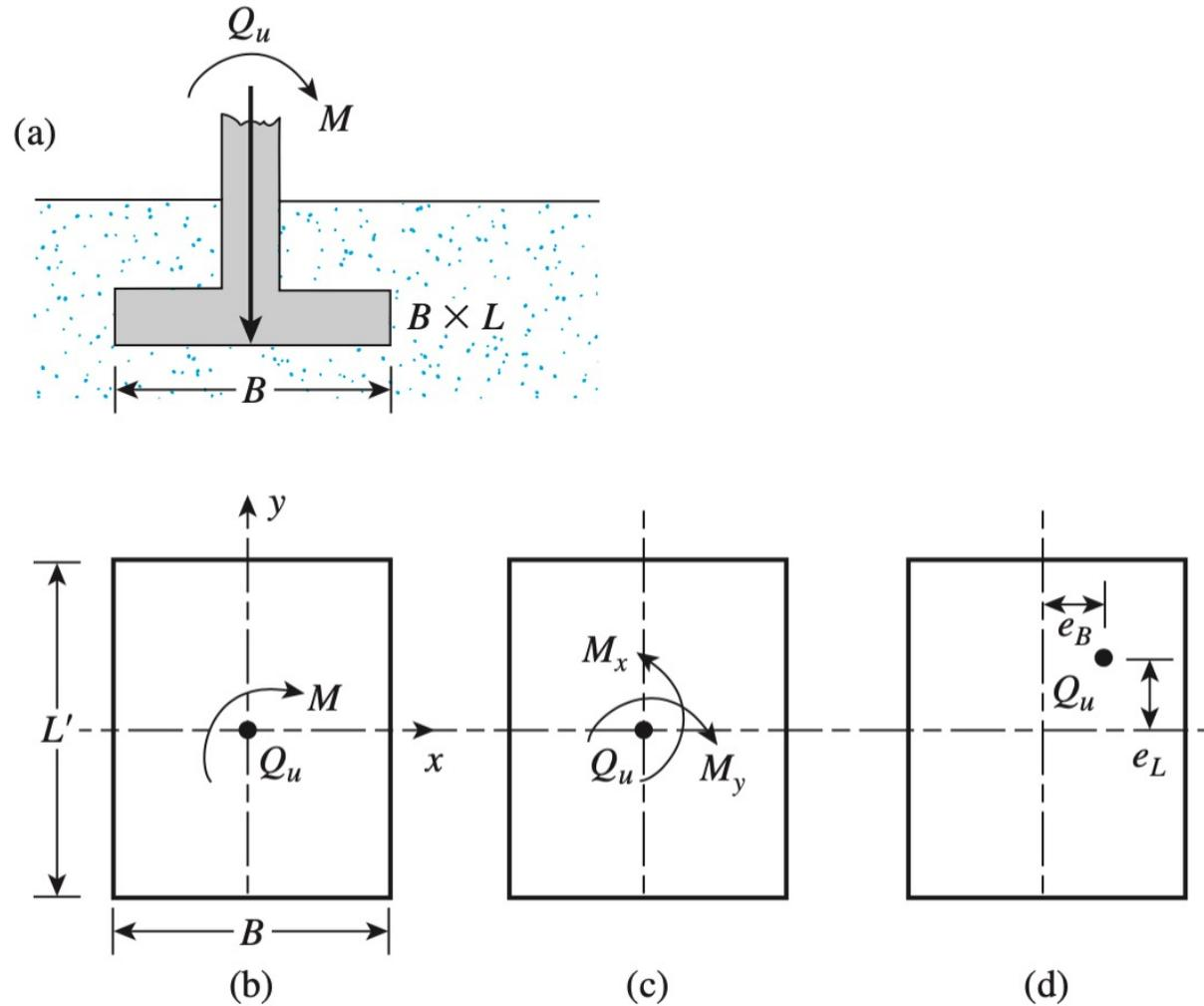
**Figure 4.24** Analysis of foundation with two-way eccentricity
