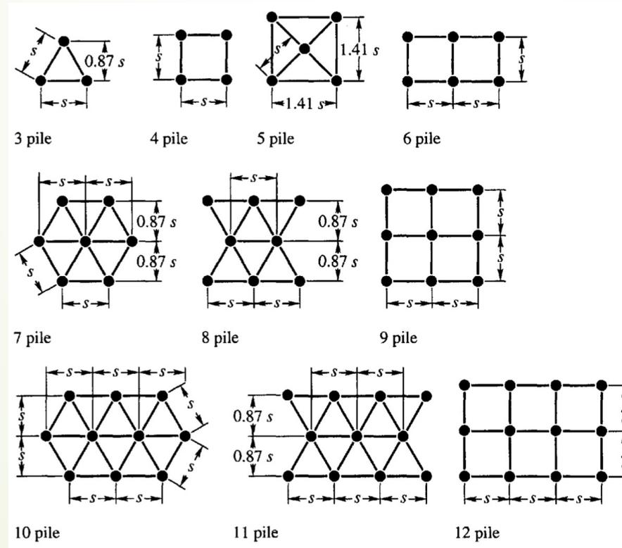
The minimum allowable spacing of piles is usually stipulated in building codes.
