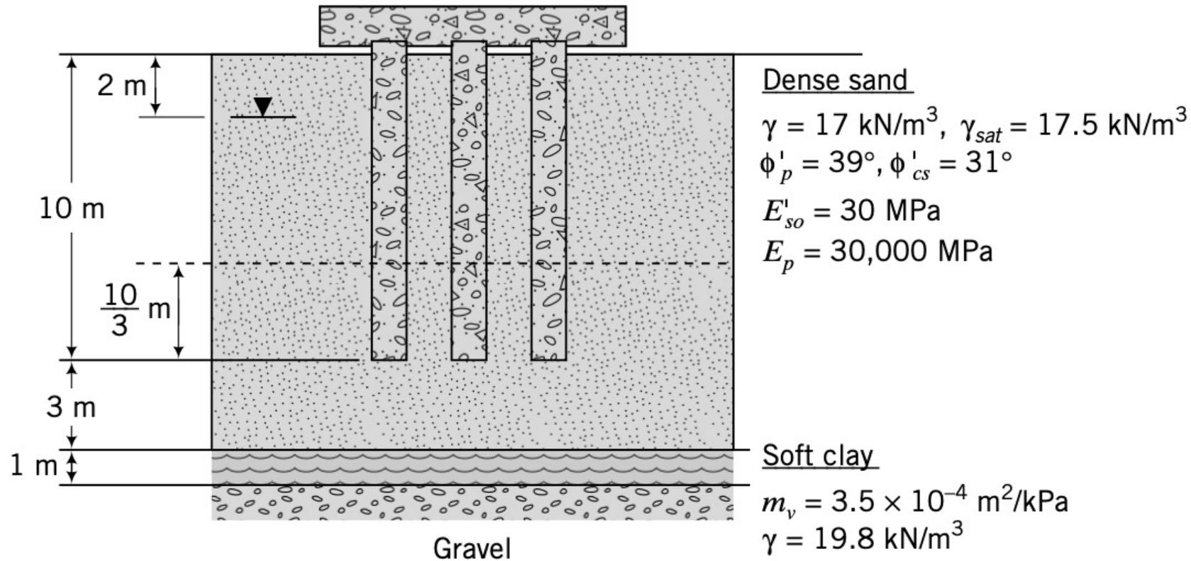
$$D = 0.4 \text{ m}, \quad \frac{L}{D} = \frac{10}{0.4} = 25; \quad n = 9 \text{ piles}, \quad s = 1 \text{ m}$$
