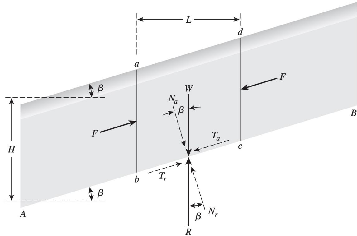
b) Analysis of infinite slope (with seepage)
