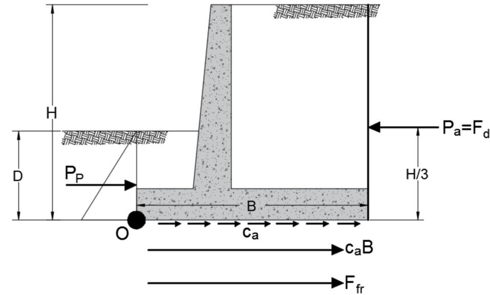
**Note:** Since there exist eccentricity, the pressure under the base of retaining wall is not uniform (there exist maximum and minimum values for pressure).
