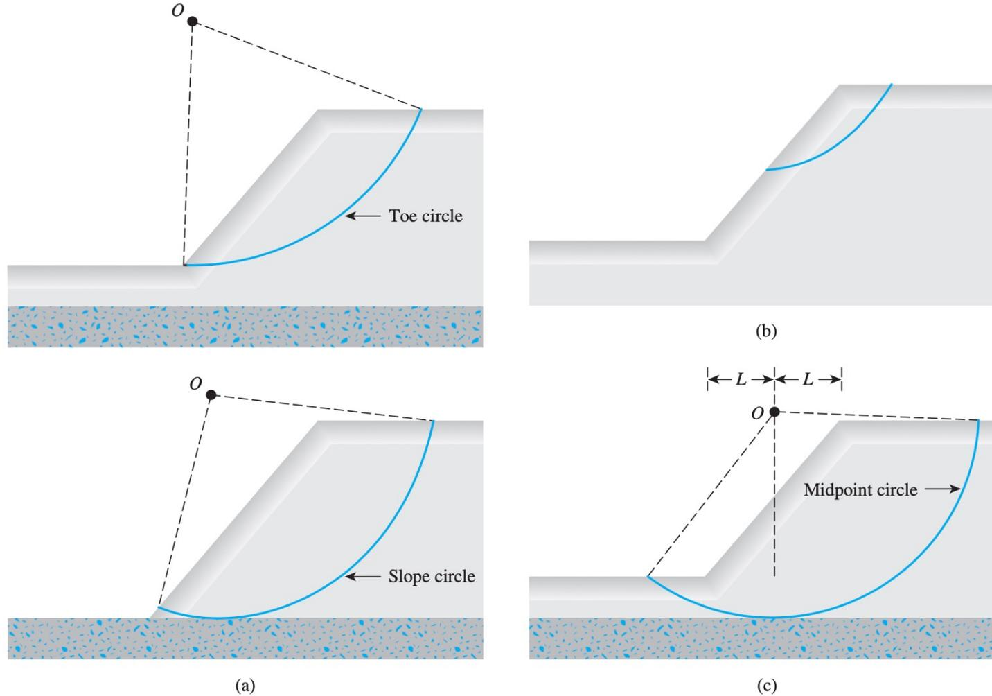
**Modes of failure of finite slope:** (a) slope failure; (b) shallow slope failure; (c) base failure
