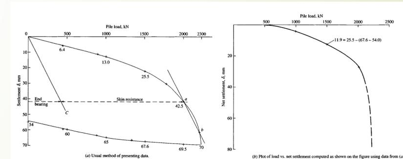
A typical results of Pile Test from (Bowels)
