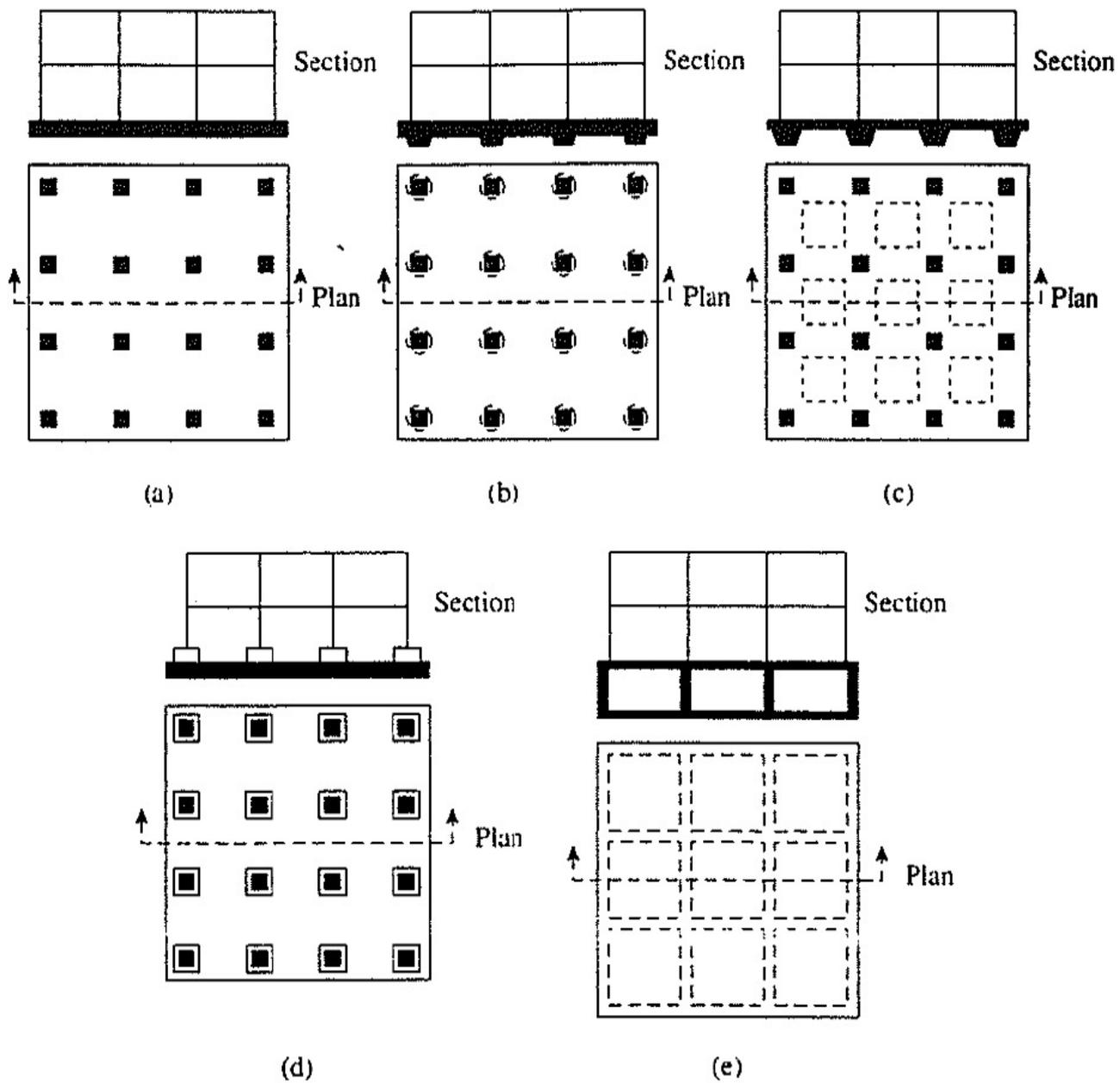
**Figure 6.4** Common types of mat foundation
