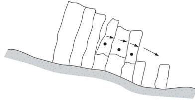
2: Slope failure by "toppling"
