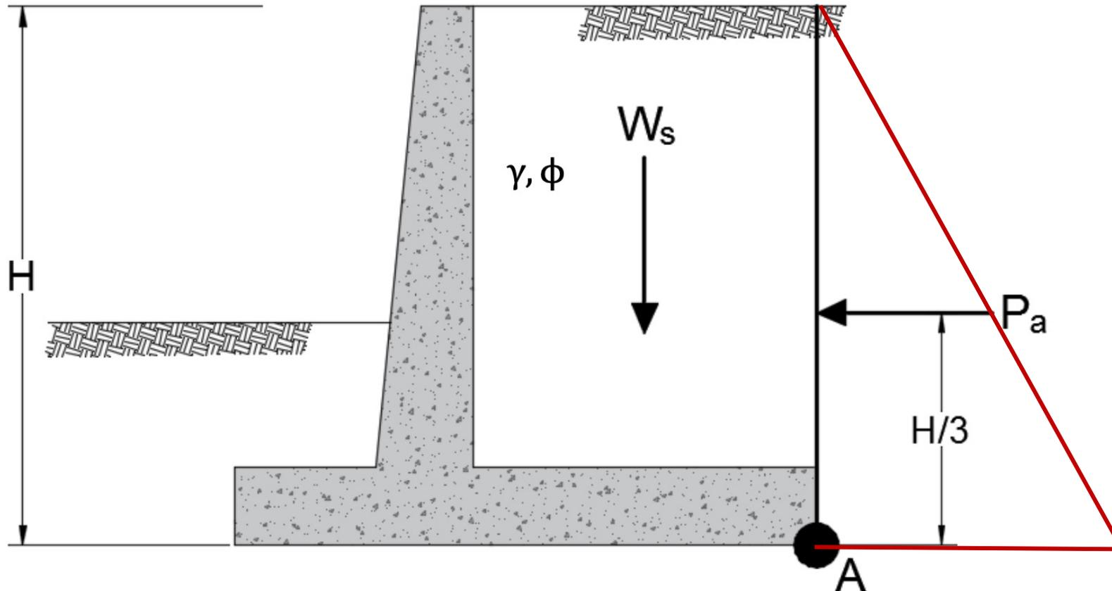
Here the active force  $P_a$  is horizontal and can be calculated as following:
