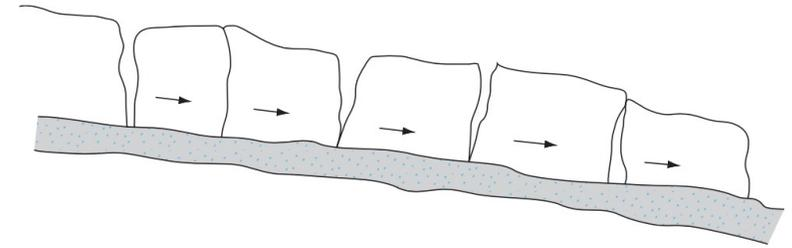
4: Slope failure by lateral "spreading"
