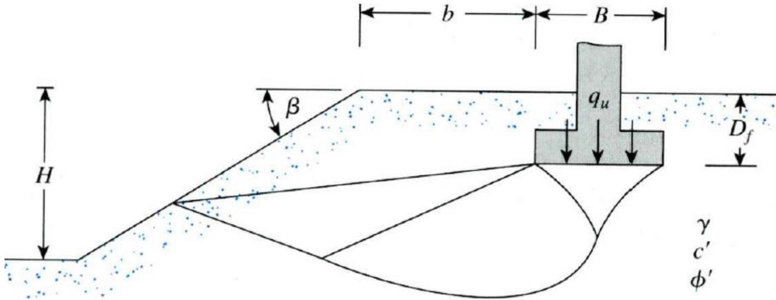
$H$  = height of slope ,  $\beta$  = angle between the slope and horizontal
