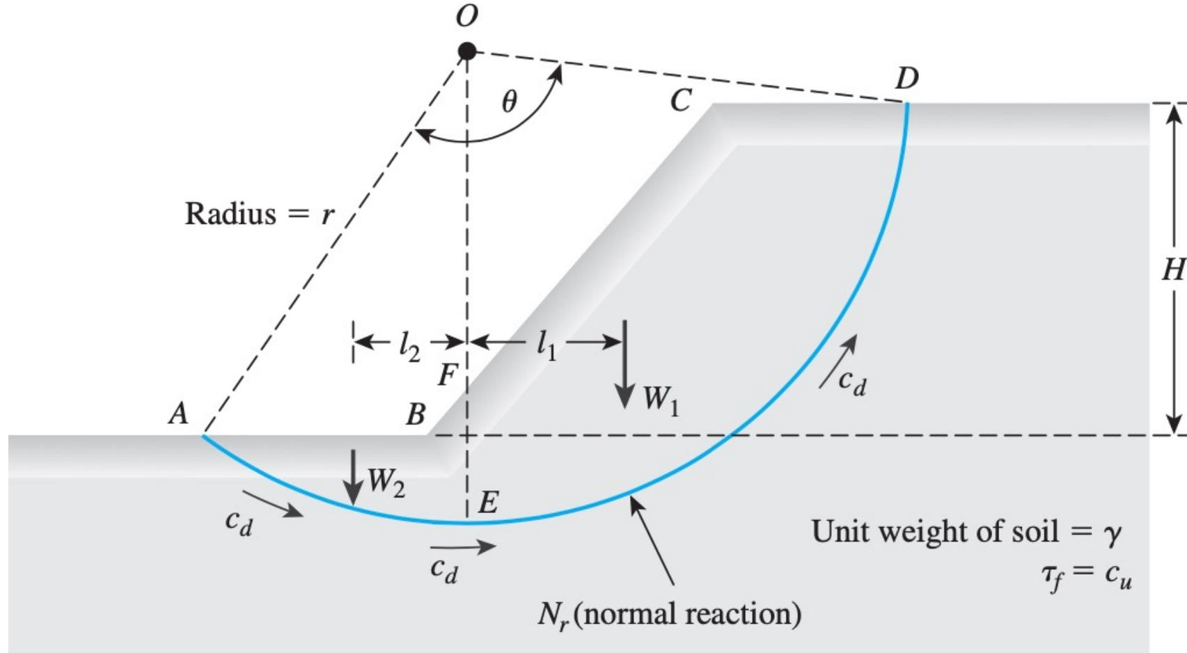
**Stability analysis of slope in homogeneous saturated clay soil**
