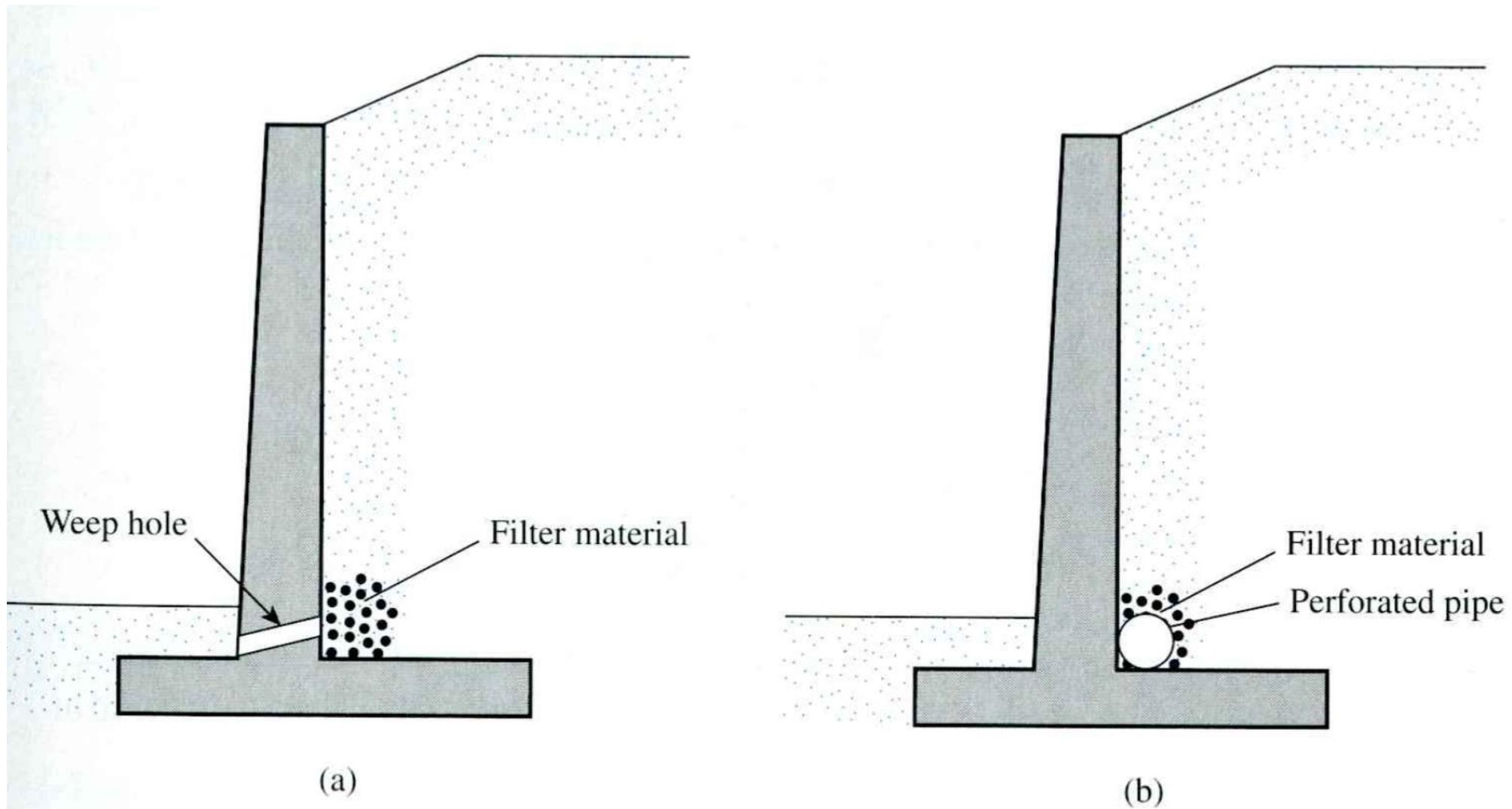
**Figure 8.15** Drainage provisions for the backfill of a retaining wall: (a) by weep holes; (b) by a perforated drainage pipe
