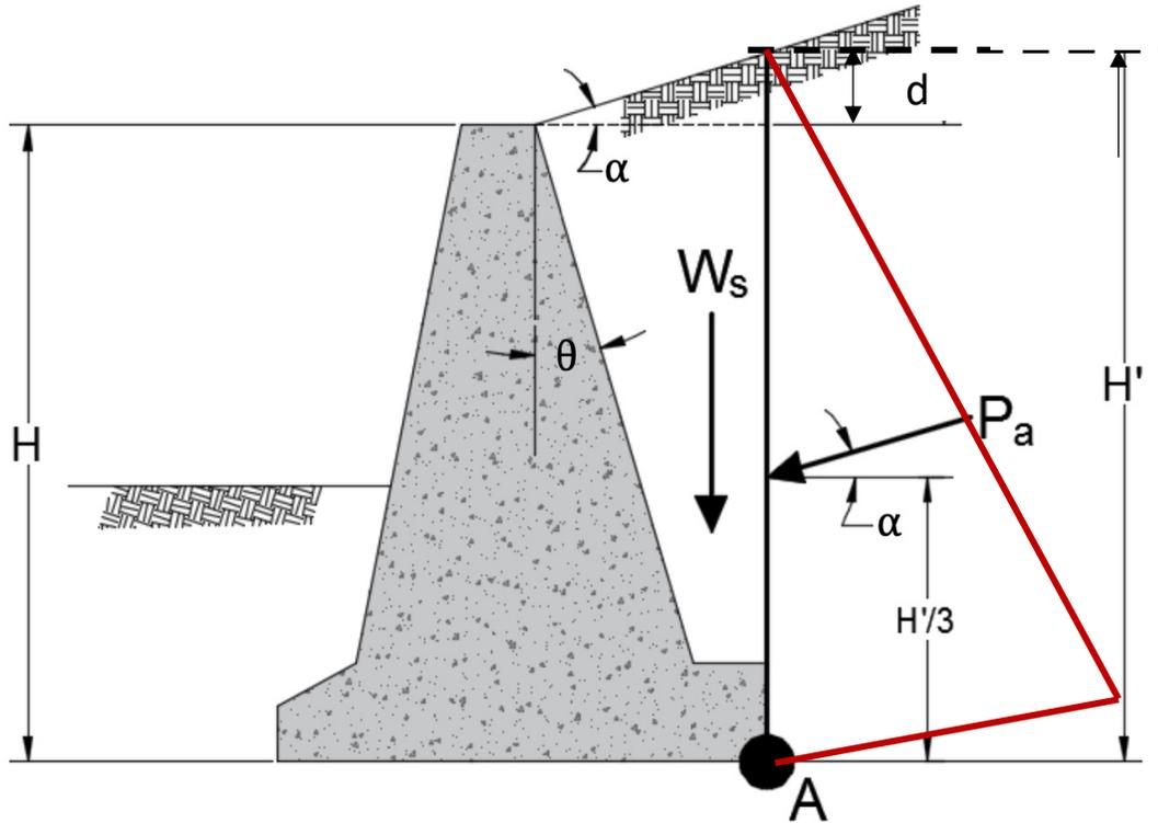
Note that the force  $P_a$  is inclined with angle ( $\alpha$ ) and not depend on the inclination of the wall because the force applied on the vertical line and can be calculated as following:
