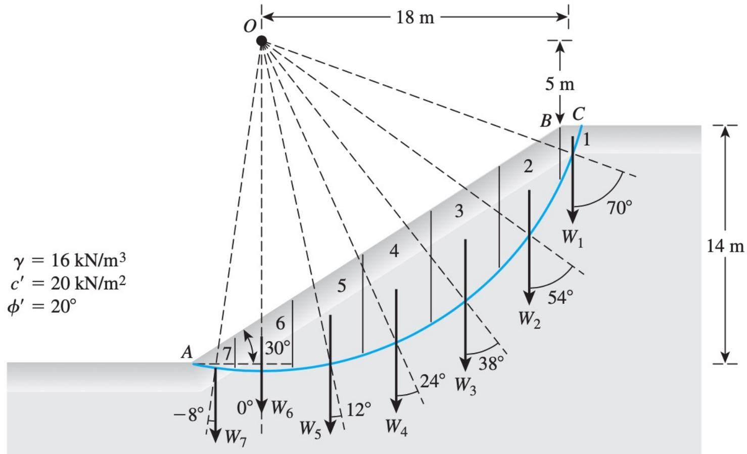
Stability analysis of a slope by ordinary method of slices
