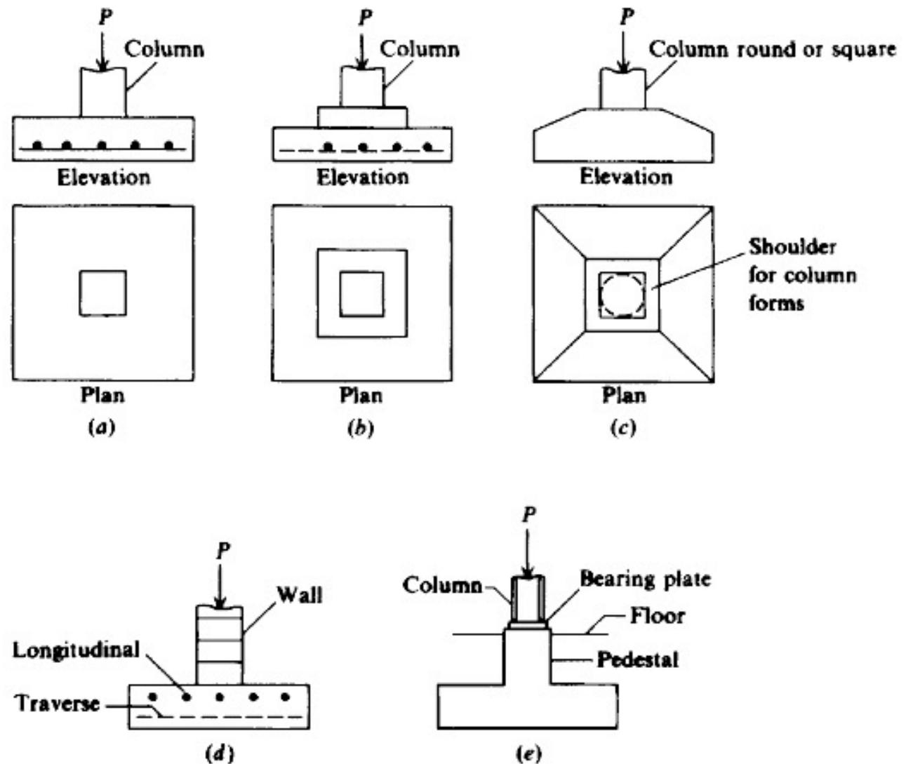
Typical footings, (a) *Single or spread footings*; (b) *stepped footing*; (c) *sloped footing*; (d) *wall footing*; (e) *footing with pedestal*.
