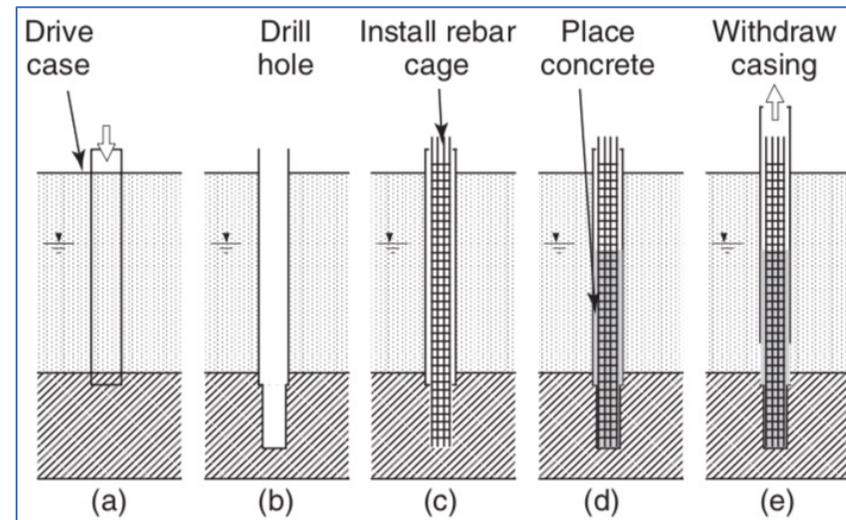
Fig. -2-: Casing method
