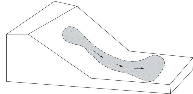
5: Slope failure by "flowing"
