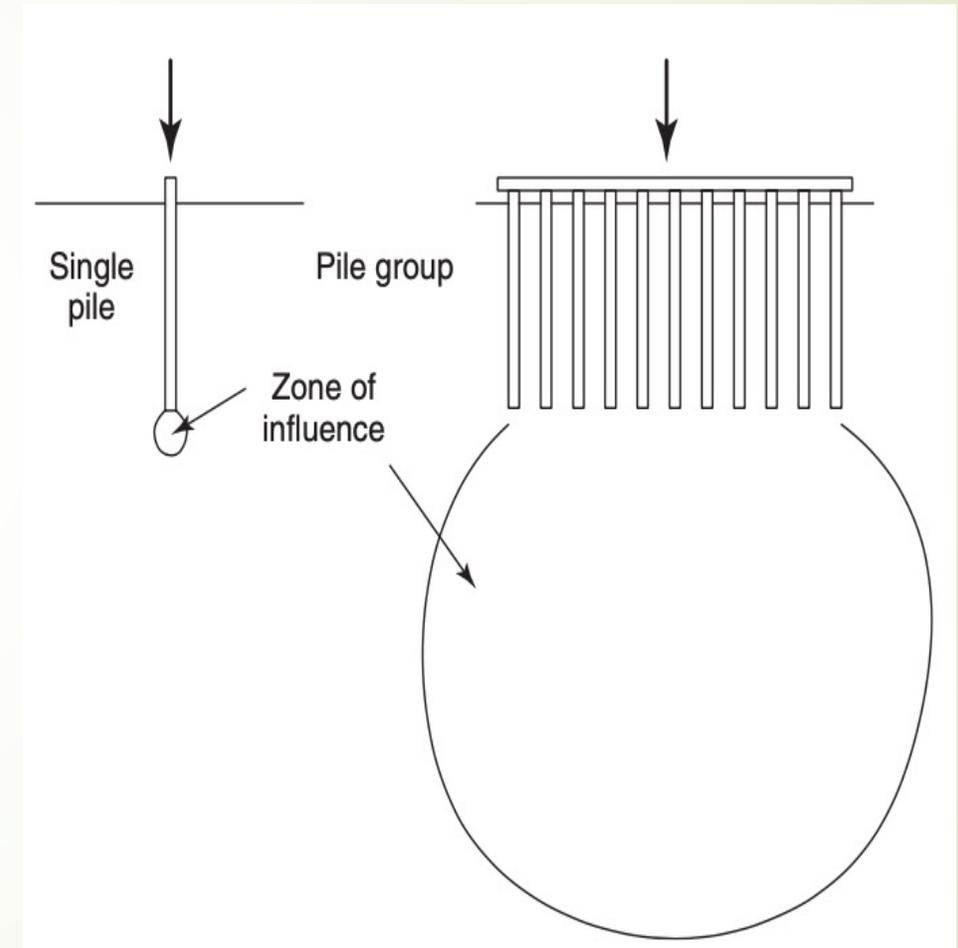
Experimental results have indicated that when a pile group installed in cohesive soils is loaded, it may fail by any one of the following ways:
