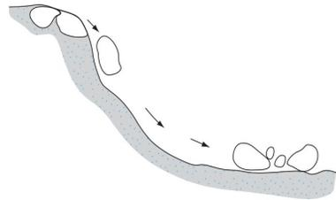
1: "Fall" type of landslide
