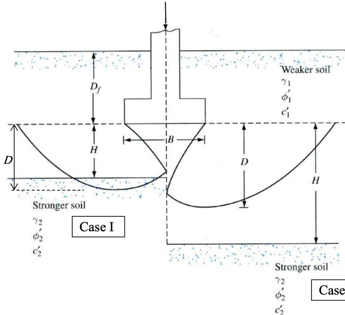
Because failure surface is fully located on top (weaker soil).
