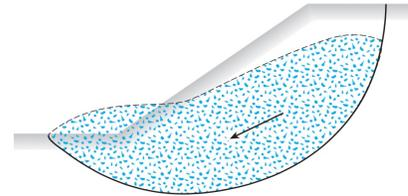
3: Slope failure by "sliding"
