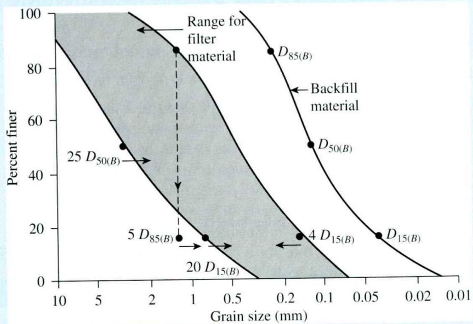
**Figure 8.16** Determination of grain-size distribution of filter material
