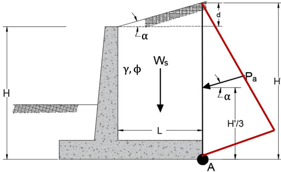
Here the active force  $P_a$  is inclined with angle ( $\alpha$ ) and can be calculated as following:
