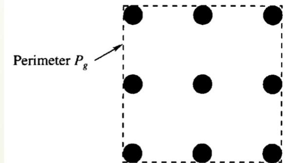
The bearing capacity of a pile group on the basis of individual pile failure may be written as
