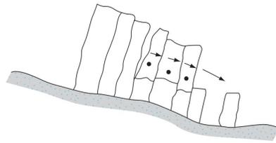
2: Slope failure by "toppling"
