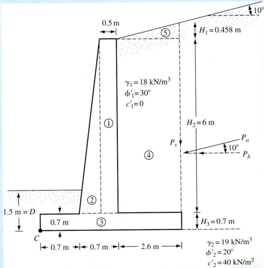
Figure 8.12 Calculation of stability of a retaining wall
