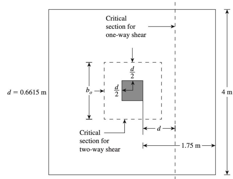
For two-way shear, the critical section is located at a distance of  $d/2$  from the edge of the column (ACI Code Section 11.11.1.2). This is shown in Figure . For this case, [with  $\lambda = 1$  in Eq.
