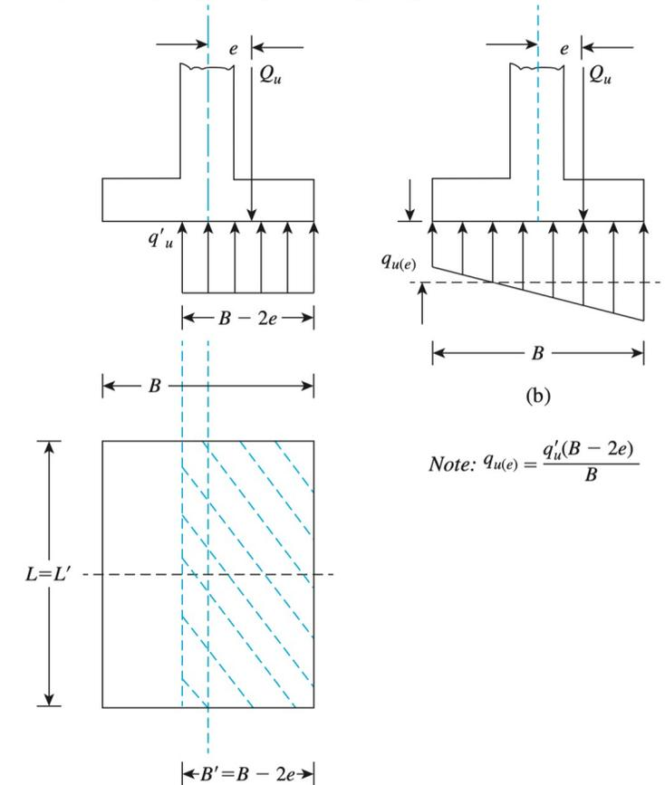
4) The factor of safety against bearing capacity failure is:  $FS = \frac{Q_u}{Q}$
