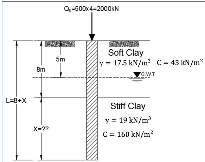
$$Q_{\text{all}} = 500 \text{ kN} , \quad \text{FS} = 4 \rightarrow Q_u = 500 \times 4 = 2000 \text{ kN}$$
