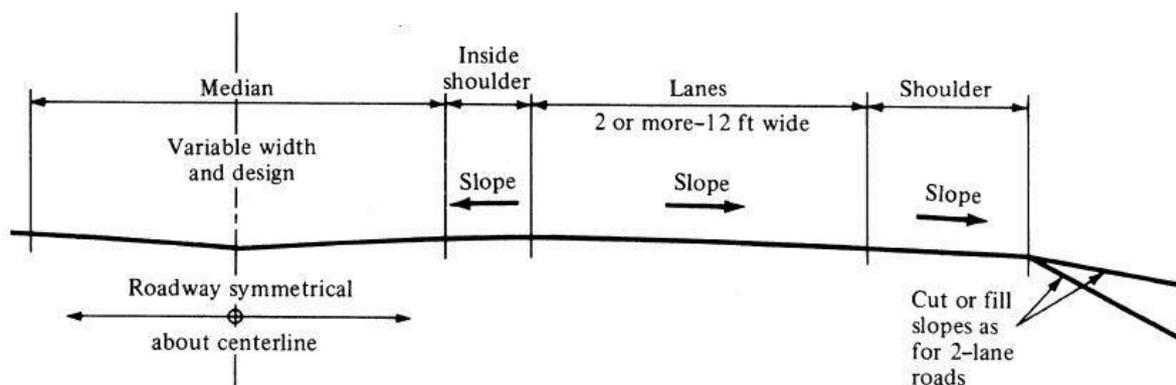
**Figure 2.2: Typical cross section of multi-lane highways**
