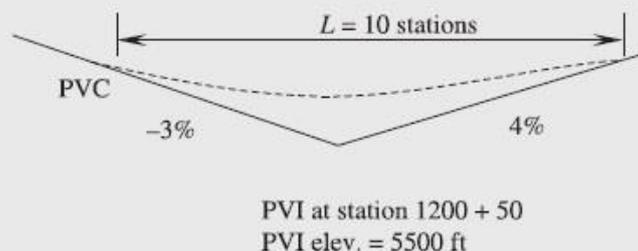
Calculate the horizontal distance to the lowest point of the sag curve, and the tangent offset at the PVI.
