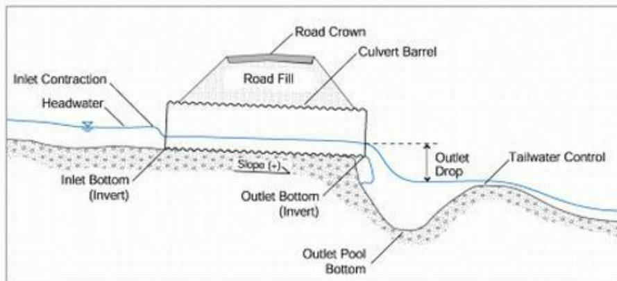
**Figure 2.5: Culvert under roadway**
