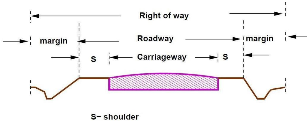
Figure 2.8: Typical right of way section
