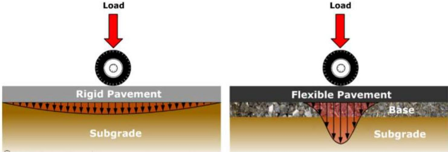
Stresses distribution under rigid and flexible pavements
