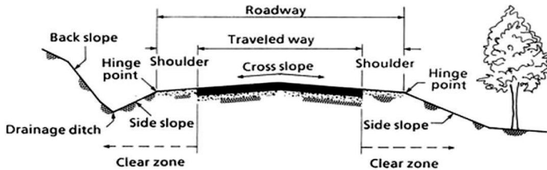
**Hinge Point** Point where the slope rate changes.
