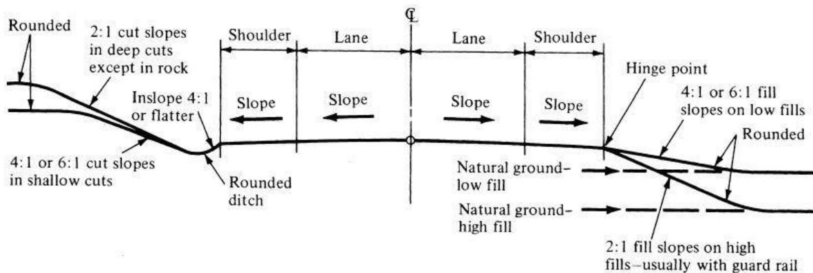
**Figure 2.1: Typical cross section of two-lane highways**
