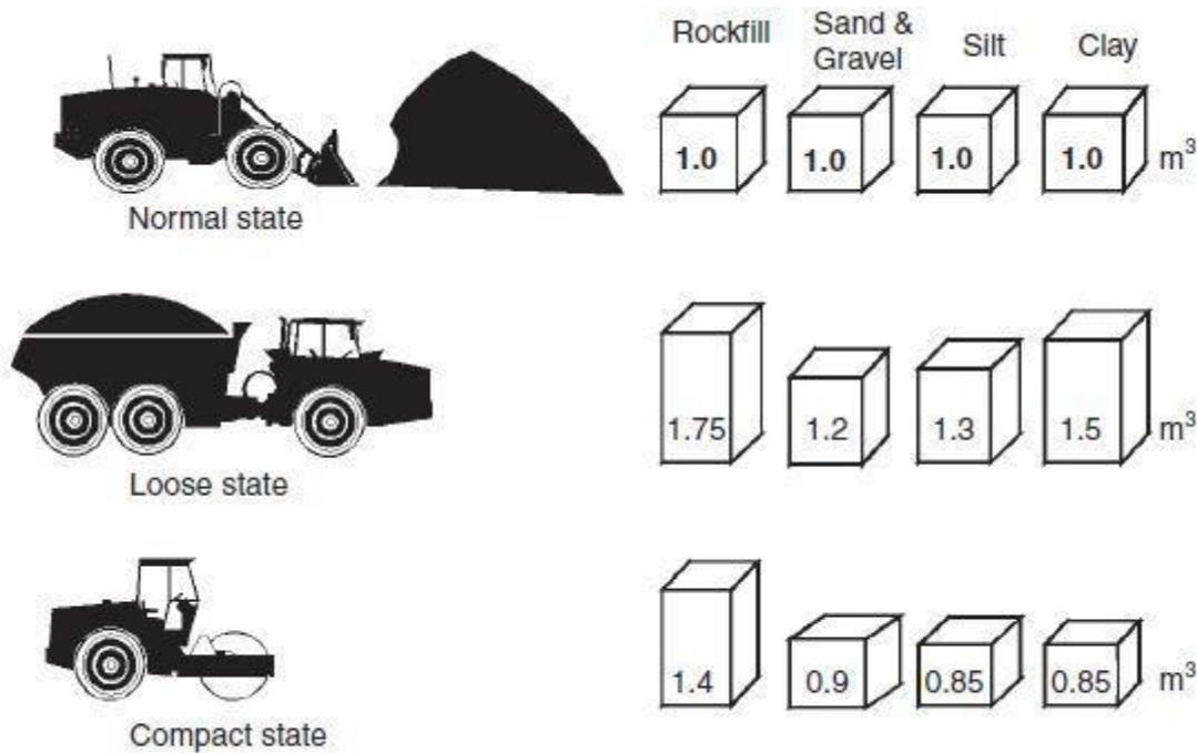
The ratio of the loose volume to the in-situ or non-excavated volume is termed the **swelling factor** or the **shrinkage factor**. These factors are applied to **the fill volume** in order to determine the required quantity of fill material.
