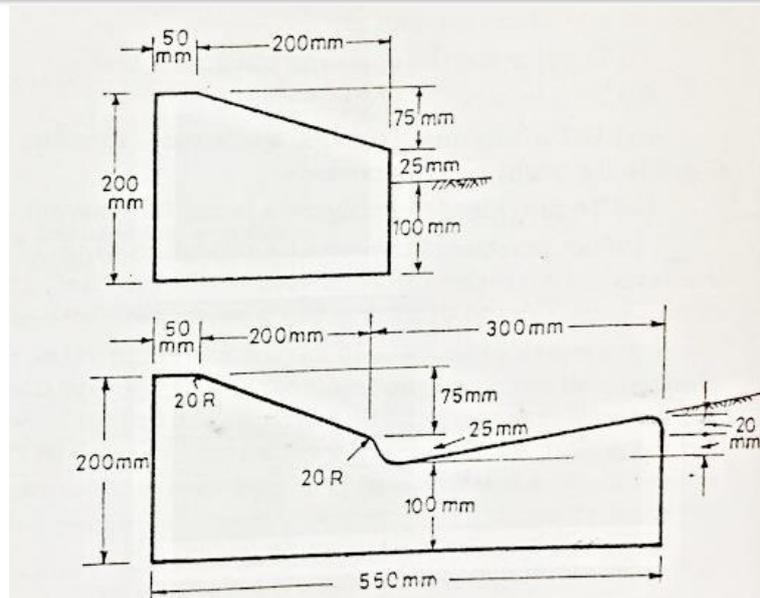
**Figure 2.3: Curb and gutter**
