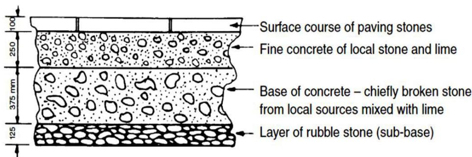
**Figure (1-1) Roman Road Structure (All dimensions in mm)**
