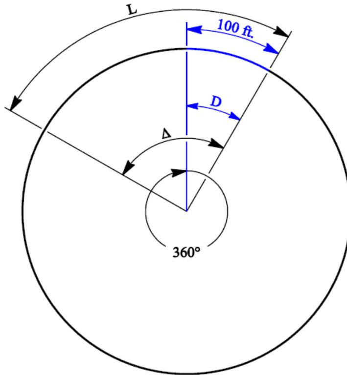
Figure 5-3: Degree of curvature
