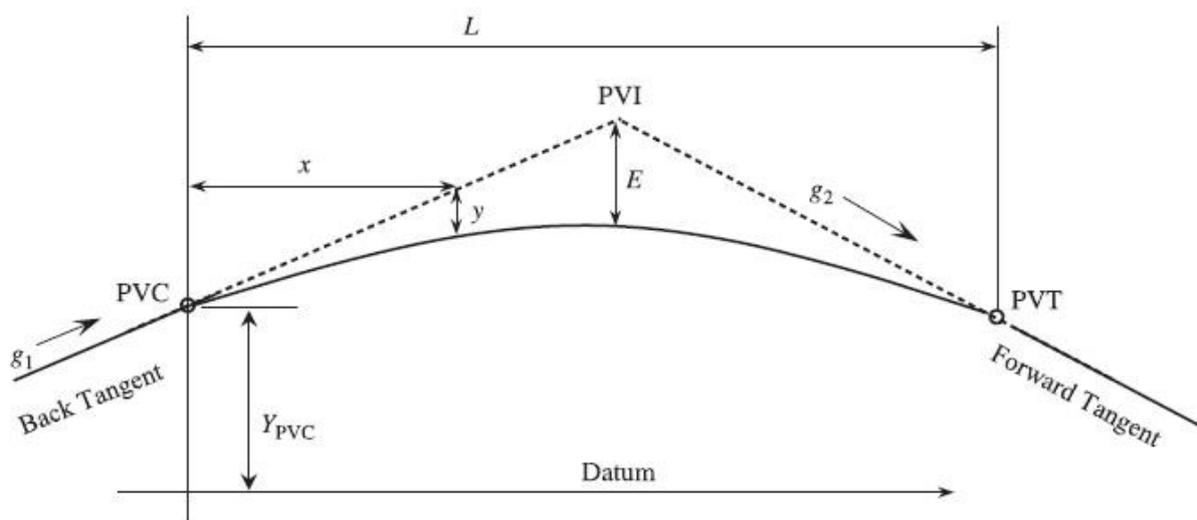
distances measured from the PVC, and  $y$  values are elevations measured from the vertical datum of reference. The following formulas can be derived from the above figure using trigonometry:
