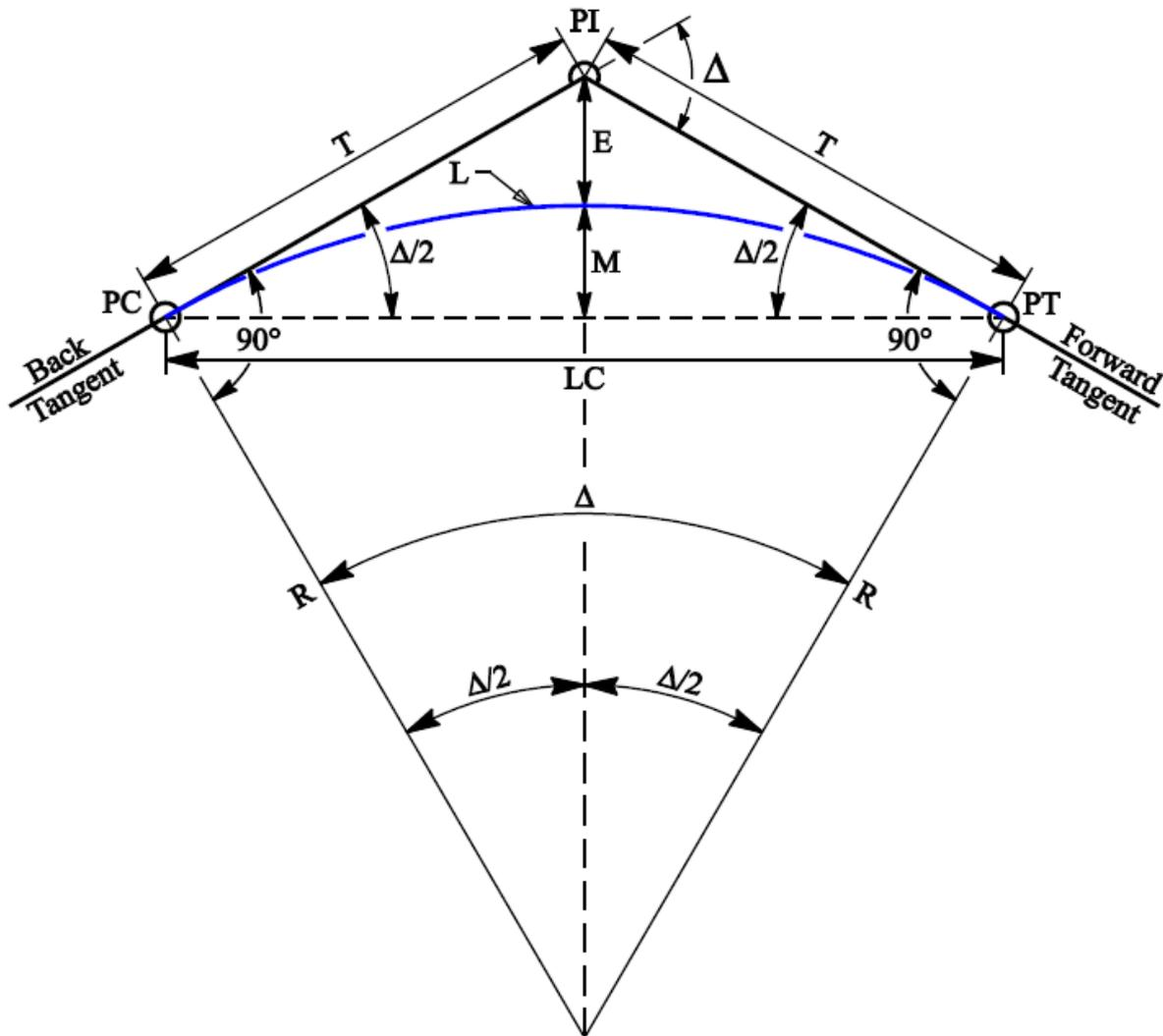
Figure 5-2: Circular curve components
