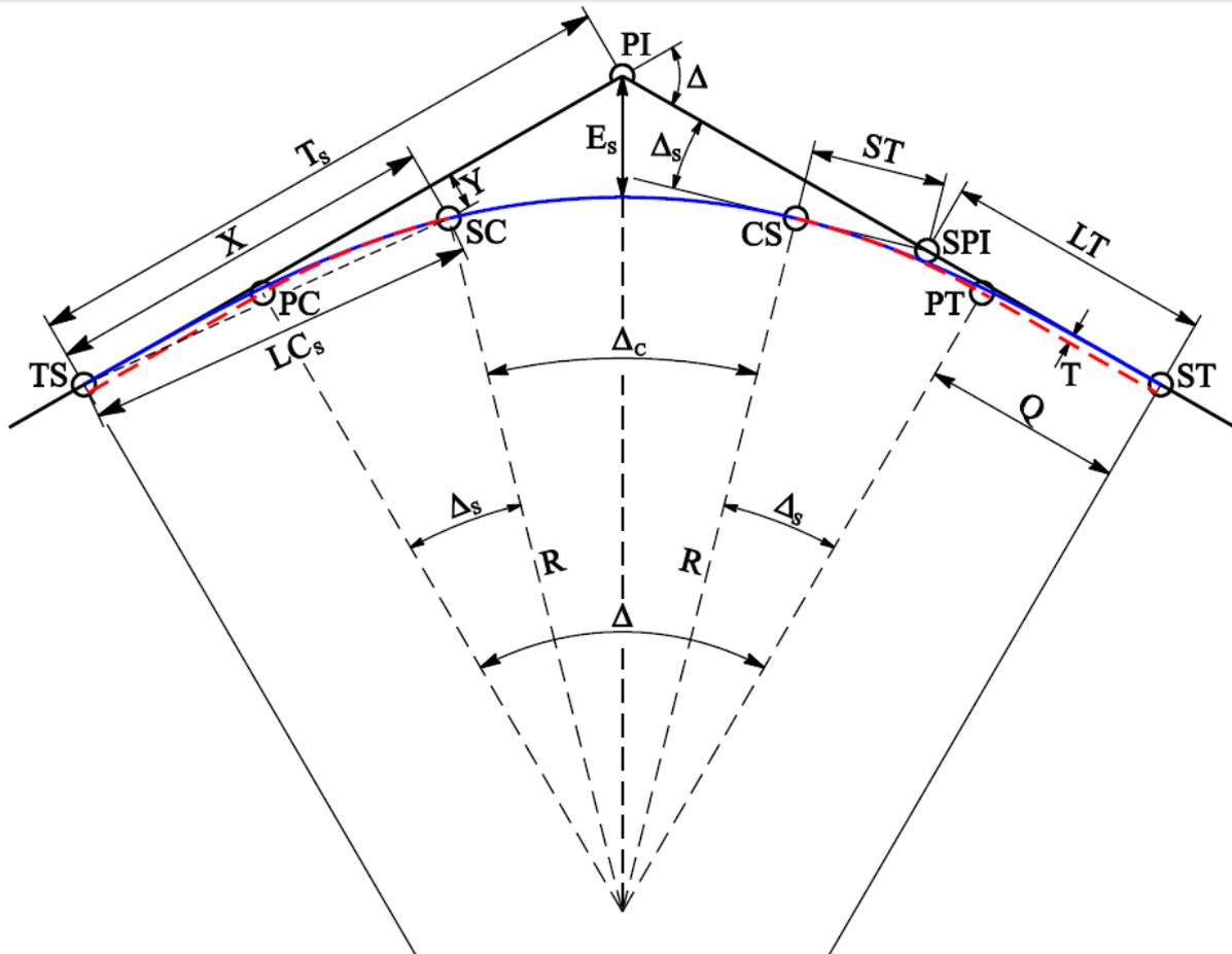
**Figure 5-1: Spiral curve components**
