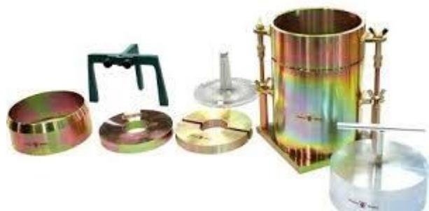
$$\text{CBR} = \frac{\text{(unit load for 0.1 piston penetration in test specimen) (lb/in}^2\text{.)}}{\text{(unit load for 0.1 piston penetration in standard crushed rock) (lb/in}^2\text{.)}} \quad (17.24)$$
