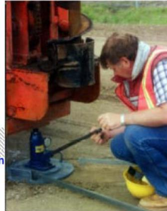
**Plate Loading Test**
