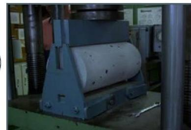
Split cylinder test specimens
