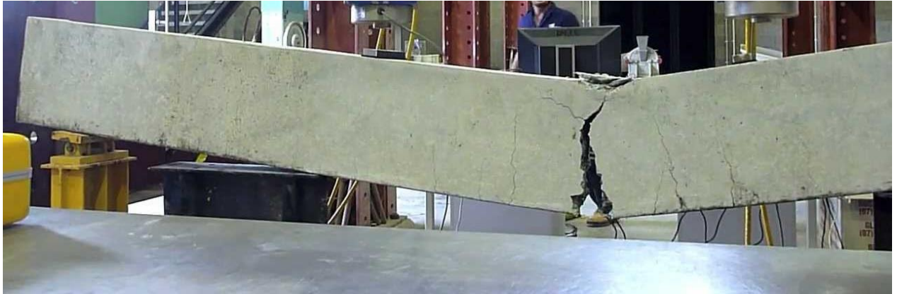
Figure (2) flexural Failure (vertical crack)
