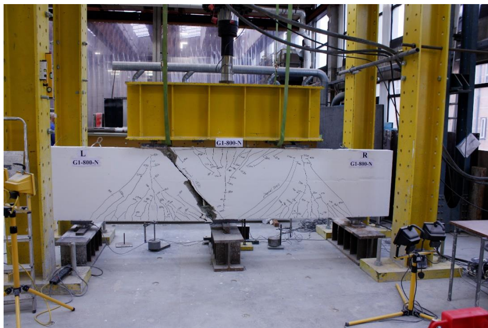
Figure (1) Shear Failure (diagonal crack)
