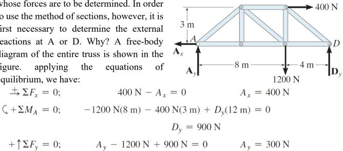
Free-Body Diagram. For the analysis, the free-body diagram of the left portion of the sectioned truss will be used, since it involves the least number of forces.
