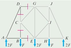
In the figure, we obtain a section by cutting members DG, CD, BC, and BE. Because the lines of action of  $T_{BE}$ ,  $T_{BC}$ , and  $T_{CD}$  pass through point B, we can determine  $T_{DG}$  by summing moments about B:
