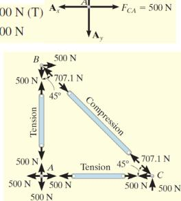
**Example 2:** Determine the force in each member of the loaded truss. Make use of the symmetry of the truss and of the loading.
