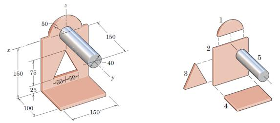
**Solution**. The composite body may be considered to be composed of the five elements shown in the figure below. The triangular part will be taken as a negative mass. For the reference axes indicated, it is clear by symmetry that the x-coordinate of the center of mass is zero.
