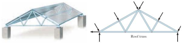
Simple trusses are composed of triangular elements. The members are assumed to be pin connected at their ends and loads applied at the joints.
