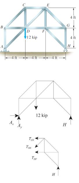
Example: Determine the axial forces in members DG and BE of the truss.
