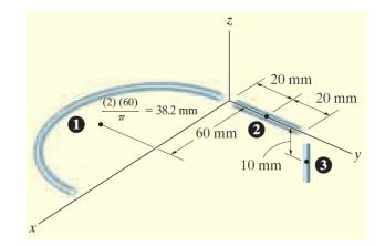
Example: Locate the center of mass of the bracket-and-shaft combination. The vertical face is made from sheet metal which has a mass of 25 kg/m2. The material of the horizontal base has a mass of 40 kg/m2, and the steel shaft has a density of 7830 Kg/m3. (All dimensions in the figure are in millimeters)
