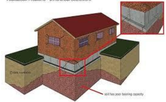
Foundation Problems - Differential Settlement
