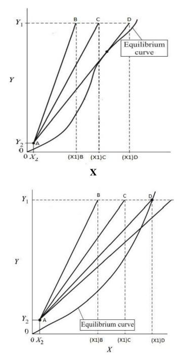
Refer to the operating line in the above figures, the slope equals to  $(L'_m / G'_m)$  and starts from the fixed point  $(X_2, Y_2)$  (point A). As the amount of solvent is gradually decreased, the slope of the operating line decreases and it comes closer to the equilibrium curve. The driving force will decrease as a result, and the larger height of packing, or a larger number of plates has to be used to achieve the desired degree of separation.
