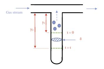
Mass transfer in the vertical tube will take place by molecular diffusion alone. Rate of evaporation can be determined by noting the change in the liquid level in the vertical tube for a particular period of time. Equation used for this method can be derived as follows:
