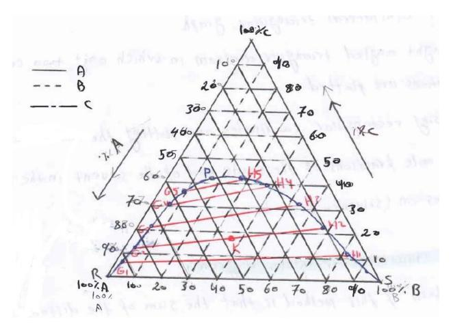
This plot represent equilibrium data for type I ternary system (C is miscible with both A and B, but A and B are partially miscible). The curve RPS is the equilibrium diagram on the equilateral triangular coordinate system. It can be constructed by plotting the data points representing the two liquid phases in equilibrium.
