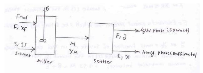
The feed that contains the solute that desired to be separated and the solvent used for separation enter the mixer in which intensive mixing occurs to attain liquid-liquid dispersion to produce a rate of M with concentration of  $x_M$  leaving the mixer towards the settler in which the produced mixture is allowed to separate into two phases. These two phases will be withdrawn separately from the settler.
