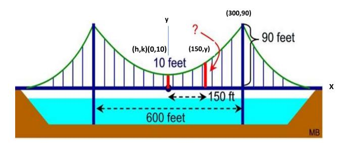
ANSWER: Let the *x*-axis be the road and the *y*-axis be the location halfway between the pillars. The vertex of the parabola will be (0,10). The point on the pillar (300,90) lies on the parabola. We need an equation for the parabola to find (150,y) on the parabola.
