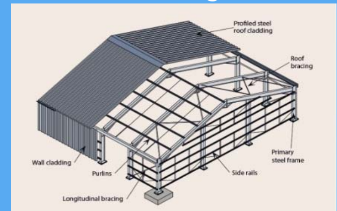
side sheeting rails
