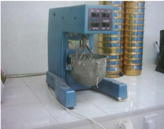
(Fig. 14 )The mixer to be used to mix the mortar
