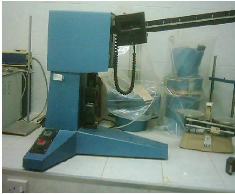
(Fig.16) The testing machine for cement mortar specimens in tension.
