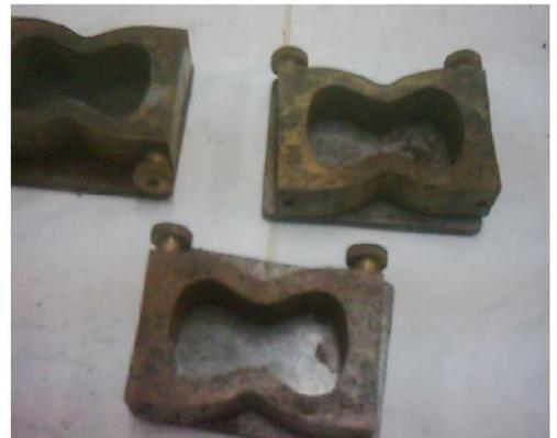
(Fig.17) The briquette molds.
