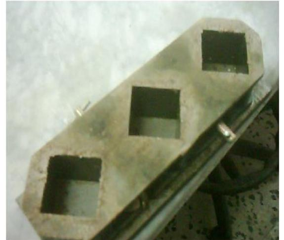
(Fig.15) The specimens molds
