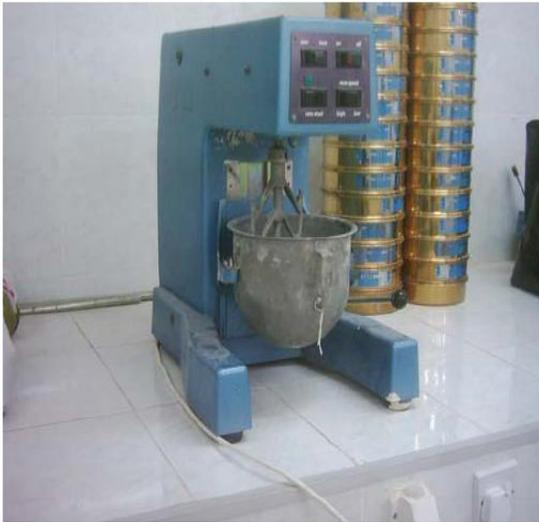
(Fig. 14 )The mixer to be used to mix the mortar
