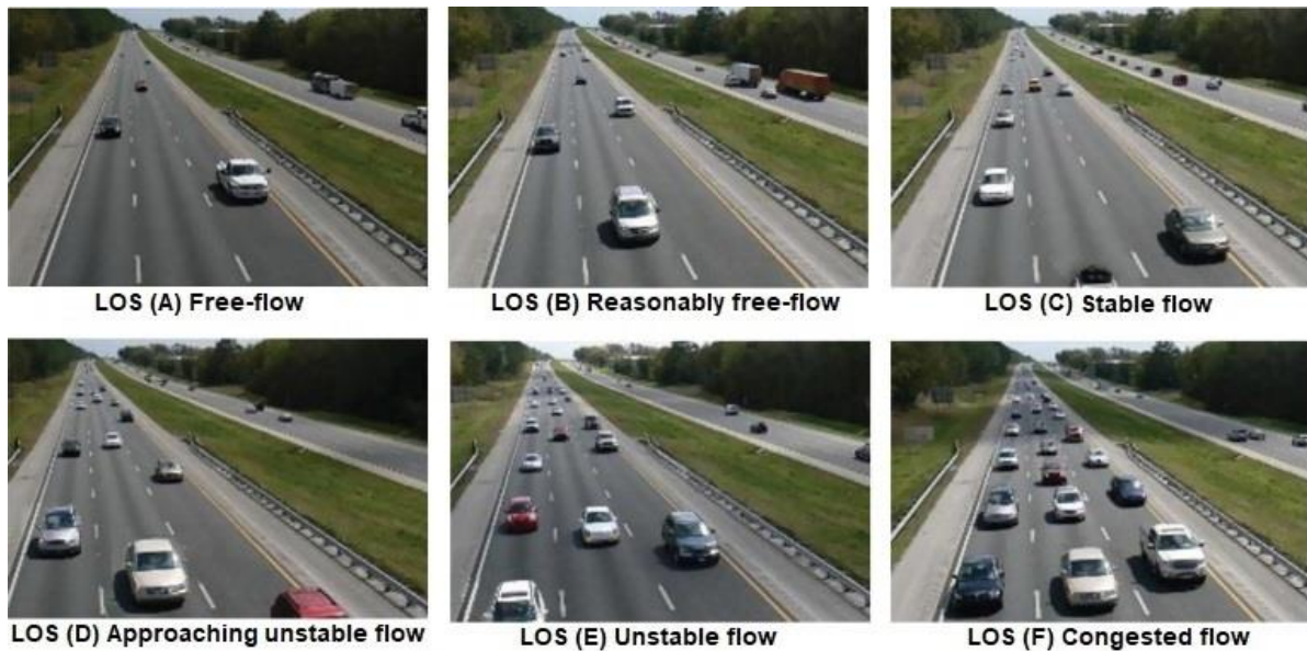
Figure 4: Illustration of six LOS on a highway
