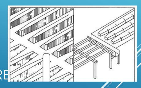
STRUCTURES RIBBED SLAB SYSTEM
