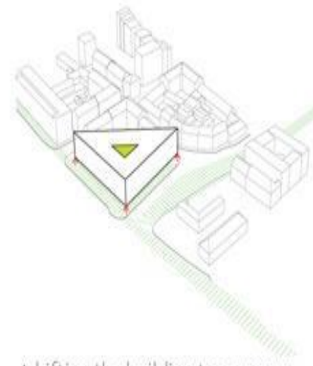
4. Lifting the building to preserve the Roman Ruins.
